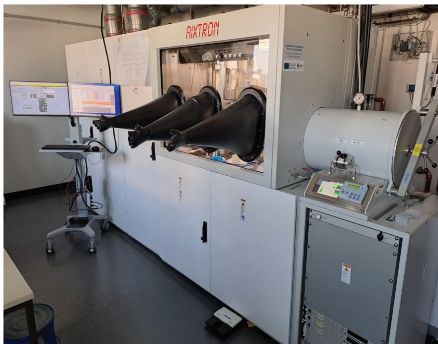
➤ The Aixtron CCS system with which NextGO Epi produces its Ga 2 O 3 epiwafers.
