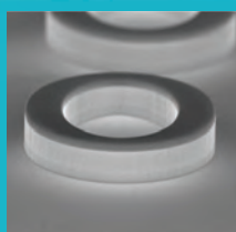
InP based material etch, vertical and smooth for maximum laser light output.
