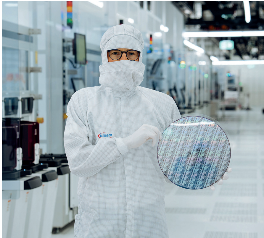
➤ A technical engineer in the cleanroom at Infineon Technologies in Villach, Austria, holds a 300 mm GaN-on-silicon wafer.
