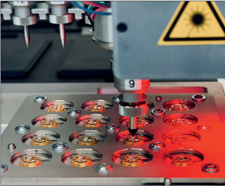
➤ Automated die bonding at Bay Photonics of customised TO-can packages for atomic clock applications.
