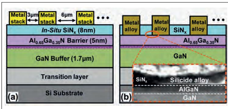
➤ After adding the metal contact to the heterostructure with a SiN layer (a), the annealing step creates a metal alloy that's in contact with the  $\text{Al}_{0.65}\text{Ga}_{0.35}\text{N}$  barrier (b).
