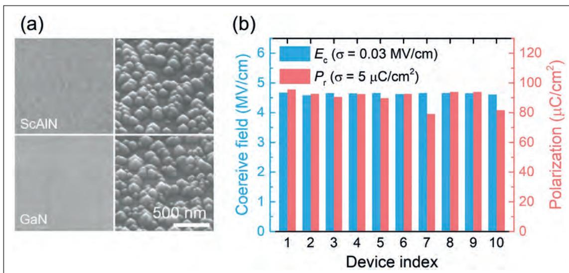
► Figure 3. (a) Scanning electron microscopy (SEM) images of as-grown (left panel) and wet chemical etched (10 wt. TMAH at 50 °C for 5 min, right panel) surface morphology for an N-polar ScAlN epilayer (upper panel) and a GaN buffer (lower panel). All SEM images share the same scale bar. (b) Coercive field and remnant polarization measured in 10 randomly distributed ferroelectric N-polar ScAlN/GaN capacitors. Taken from P. Wang *et al.* Appl. Phys. Lett. 121 023501 (2022).
