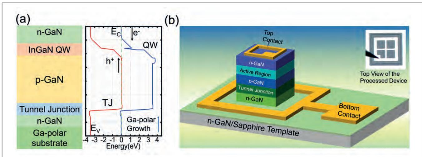
➤ Figure 2. (a) Equilibrium band diagram of the *p*-down LED using a bottom tunnel junction. (b) The finished/processed device.
