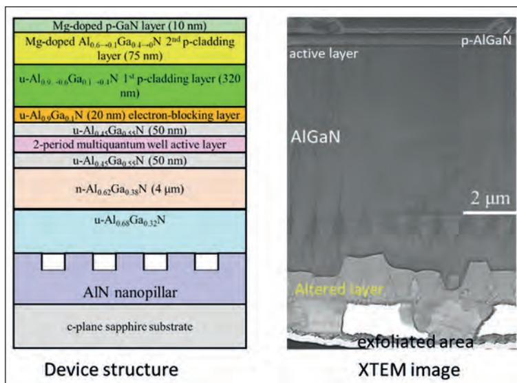
➤ A cross-sectional transmission electron microscopy image of the AlGaN-based heterostructure indicates that exfoliation takes place at the AlN nanopillar area.
