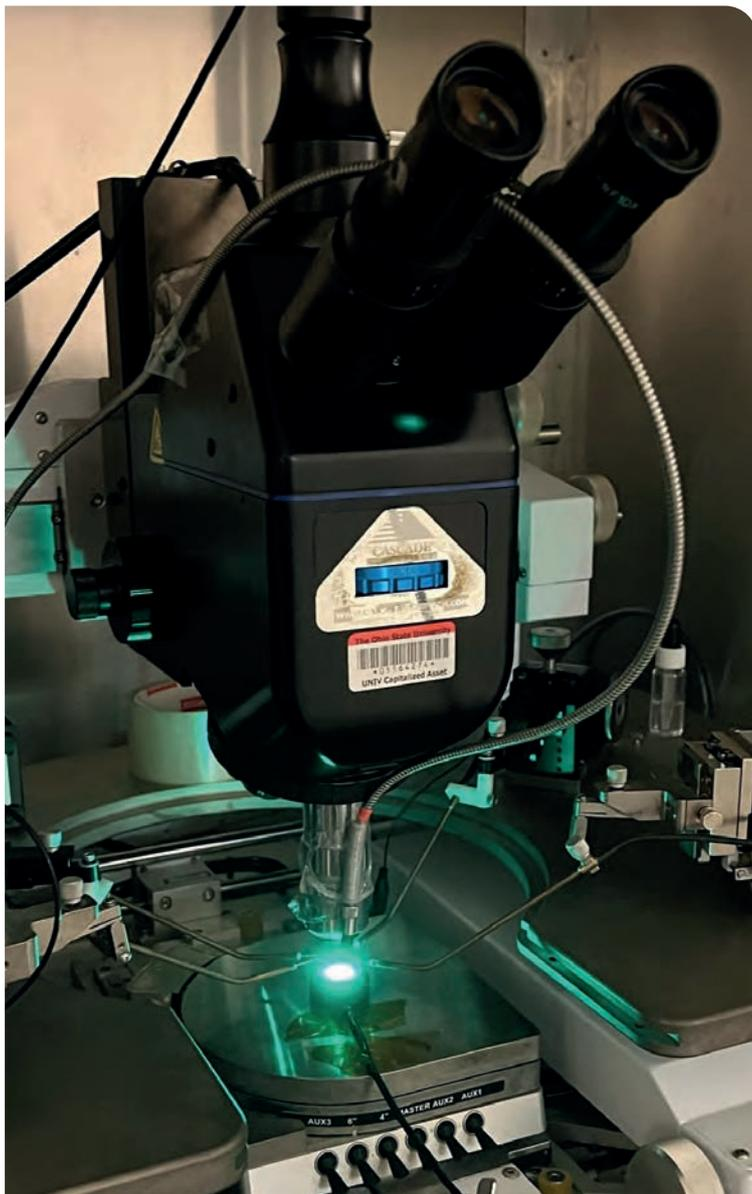
► On-wafer LED measurement set up.
