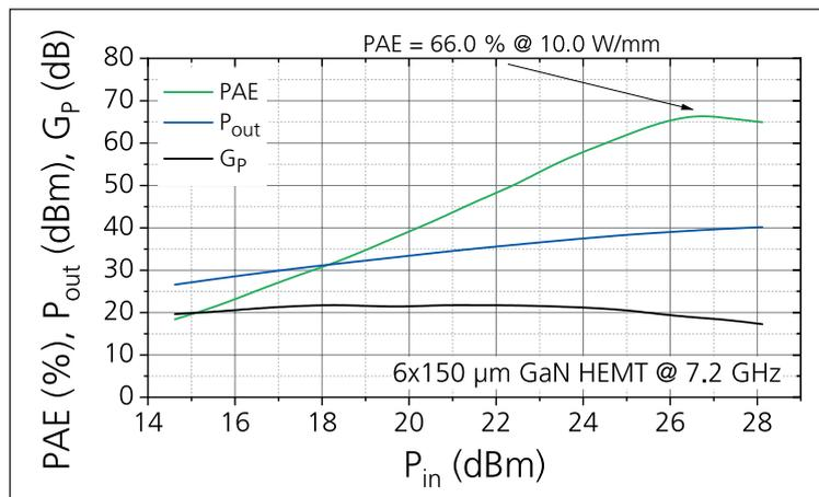
➤ Figure 4. Pulsed load-pull measurements of a 100 V GaN HEMT with a total gate width of 0.9 mm ( $6 \times 150 \mu\text{m}$ ) at 7.2 GHz. The pulse width is 100  $\mu\text{s}$ , with a duty cycle of 10 percent. For this measurement a ‘trade-off’ of fundamental impedance was chosen that yielded a good combination of efficiency and power density. Additionally, the second harmonic at the output of the device was set for the value that showed the highest power-added efficiency.
