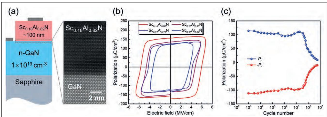
➤ Figure 1. (a) Diagram and scanning tunnelling electron microscopy image of the ScAlN/GaN interface. Taken from D. Wang *et al.* Adv. Electron. Mater. 8 2200005 (2022). (b) Polarization-electric-field loops measured at 40 kHz for ferroelectric ScAlN with varying scandium content. (c) Remnant polarization during the endurance test for  $\text{Sc}_{0.20}\text{Al}_{0.80}\text{N}$  using 10  $\mu\text{s}$  pulse width. Taken from P. Wang *et al.* Appl. Phys. Lett. 118 223504 (2021)
