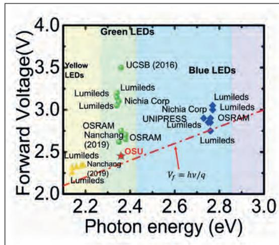
► Figure 4. Benchmark plot showing the forward-voltage drop at 20 A cm<sup>-2</sup> or 35 A cm<sup>-2</sup> for III-nitride LEDs from blue to yellow. The red line represents the lowest theoretical voltage drop,  $V_f = hv/q$ , where  $hv$  is the photon energy and  $V_f$  is the forward voltage.
