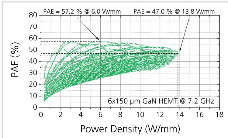
► Figure 3. Pulsed load-pull measurements of a 100 V GaN HEMT with a total gate width of 0.9 mm (6x150  $\mu\text{m}$ ) at 7.2 GHz. The pulse width is 100  $\mu\text{s}$ , with a duty cycle of 10 percent. No harmonics have been terminated during the measurement.
