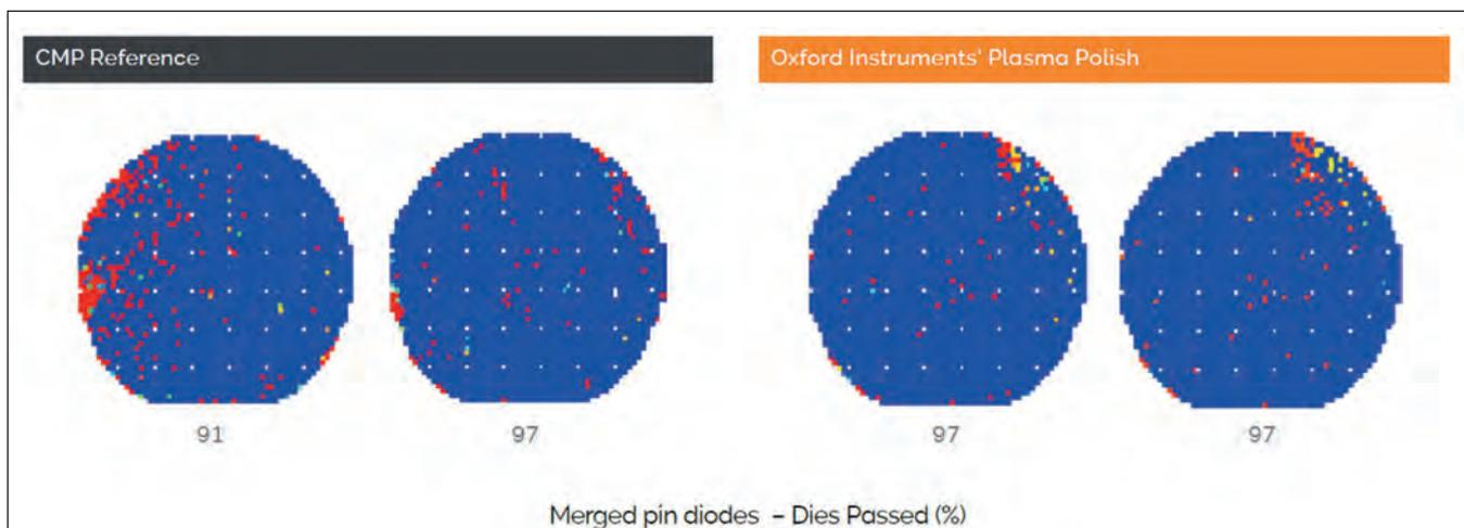
➤ Yield data highlights that the Plasma Polish process developed by Oxford Instruments delivers a device yield of SiC merged *p-i-n* diodes that is at least as high as that resulting from CMP.
