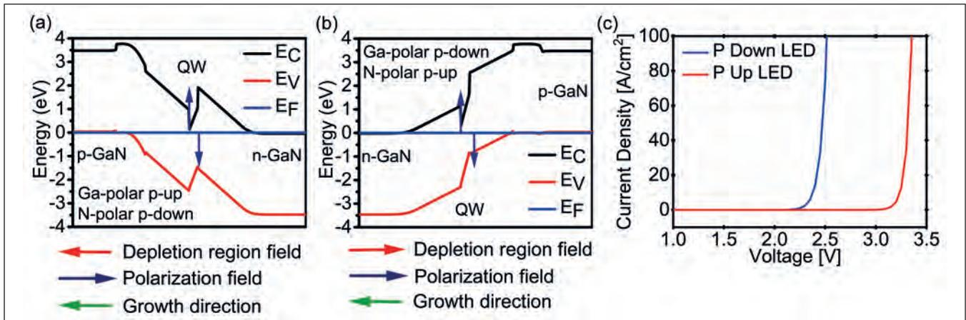
➤ Figure 1. (a), (b) Equilibrium band diagram of *p*-up and *p*-down configuration showing a low hole-injection barrier for a *p*-down design compared with a *p*-up variant; and a higher in-built electron barrier for *p*-down, improving confinement of electrons in the quantum well compared to *p*-up. (c) Simulated current density versus voltage (*J*-*V*) curve for the *p*-up and *p*-down LED structures.
