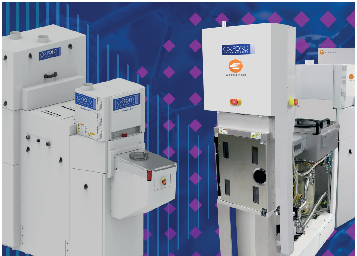
➤ Oxford Instruments Plasma Technology's PlasmaPro ASP and Atomfab suite of atomic layer deposition systems
