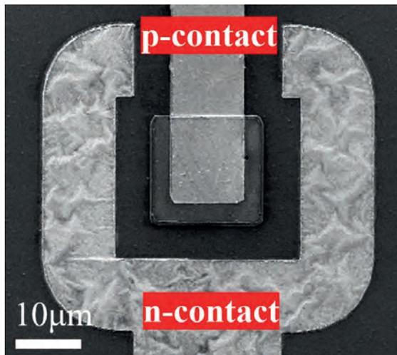
A scanning electron microscopy image of a deep-UV LED produced by UCSB that has dimensions of 20  $\mu\text{m}$  by 20  $\mu\text{m}$ .
