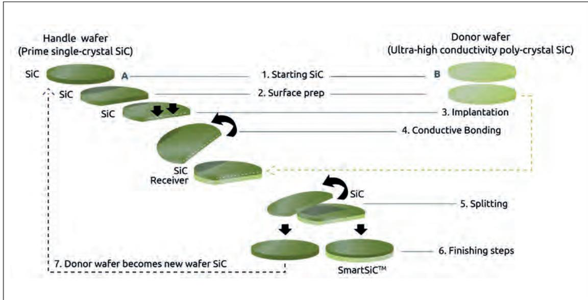
➤ Figure 2. The unique, patented Smart Cut process of Soitec, adapted to SiC material.
