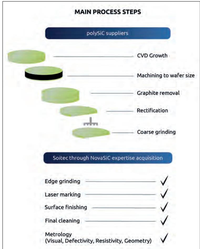
➤ Figure 3. Main process steps for manufacturing polycrystalline SiC.
