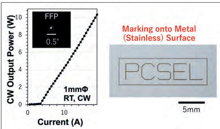
➤ Figure 10. (Left) CW operation of PCSEL with a size of 1 mm in diameter. (Right) Marking experiment onto metal (stainless) surface.
