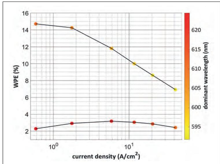
➤ Figure 5. Wall-plug efficiency (WPE) versus current density (J) for two representative encapsulated 1 mm by 1 mm InGaN red LEDs with different wavelength targets. The colour bar indicates the dominant wavelength of the emission spectrum at each point.
