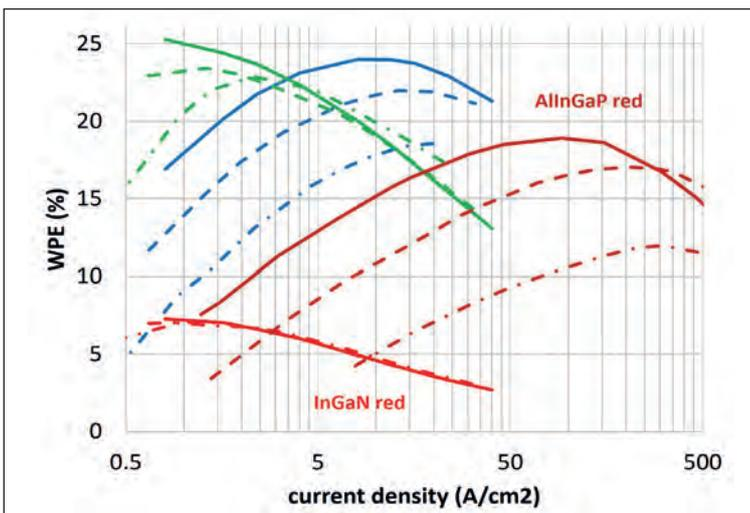
► Figure 8. Wall plug efficiency as a function of current density for microLED arrays of different colours. Solid, dashed, and dashed-dot lines indicate data in order of decreasing mesa sizes (7 µm, 4 µm, and 2 µm for InGaN; and 9 µm, 6 µm, and 4 µm for AllnGaP). The dominant wavelengths corresponding to peak efficiency are 605 nm (InGaN red), 630 nm (AllnGaP red), 540 nm (green), and 460 nm (blue).
