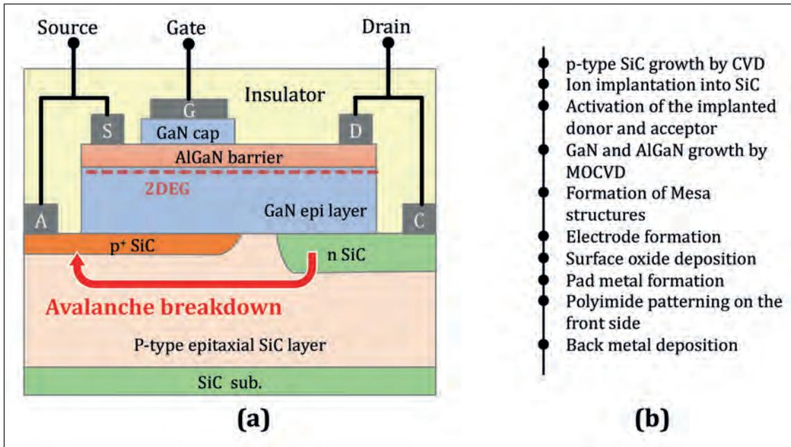
► Figure 5. (a) Schematic of a GaN/SiC-based hybrid HEMT. Five electrodes: source (S), gate (G), and drain (D) in the HEMT; and anode (A) and cathode (C) in SiC diode. (b) Our fabrication process flow for GaN/SiC hybrid HEMTs.
