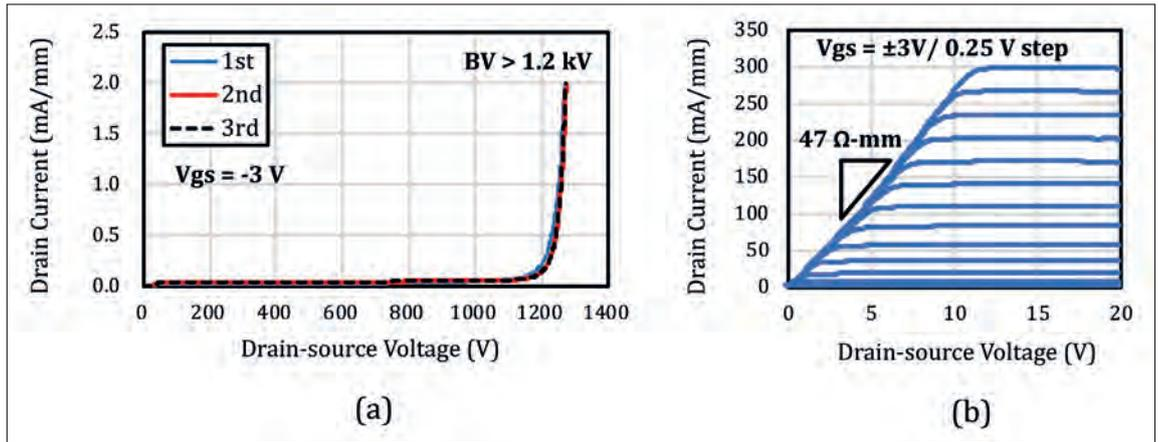
(b) On-state characteristics. Owing to current flow via the low-resistance 2DEG, a low on-resistance of 47 Ω-mm and high saturation current of 300 mA/mm were measured.
