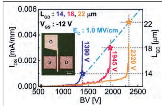
► Increasing the gate-to-drain distance of the α-Ga<sub>2</sub>O<sub>3</sub> MOSFET increases its breakdown voltage. The inset shows an optical microscopy image of the Ti/Al/Ni/Au metal gate stack.
