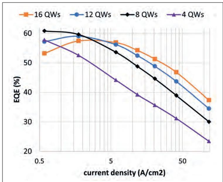
➤ Figure 2. External quantum efficiency as a function of current density for optimized green LEDs with various numbers of quantum wells in the active region.
