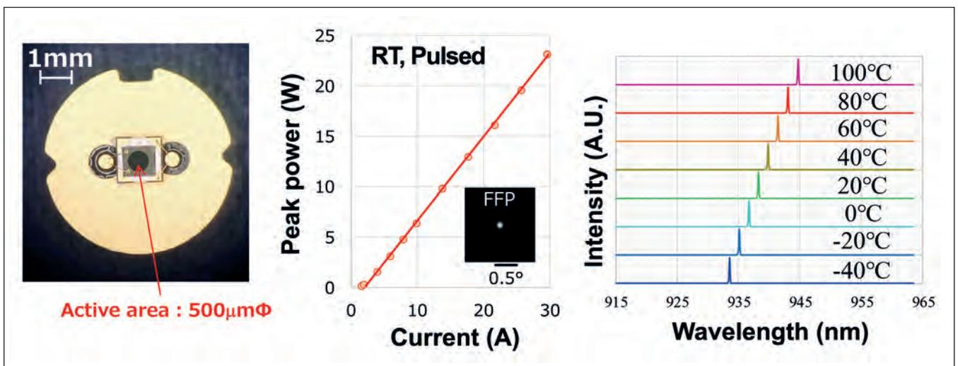
► Figure 4. (Left) PCSEL mounted on 5.6 mm-diameter package, (middle) I-L characteristic (inset shows the far-field pattern (FFP)), and (right) temperature dependence of lasing spectra.
