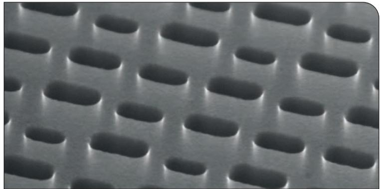
➤ Figure 11. Scanning-electron-microscope image of a dually modulated photonic crystal (bird's-eye view). Lattice-point positions and sizes are simultaneously modulated. These modulations encode information about the beam emission direction. Also, the lattice constant (equal to the spacing between the lattice points) is set to  $1/\sqrt{2}$  times the wavelength in the material (195 nm).
