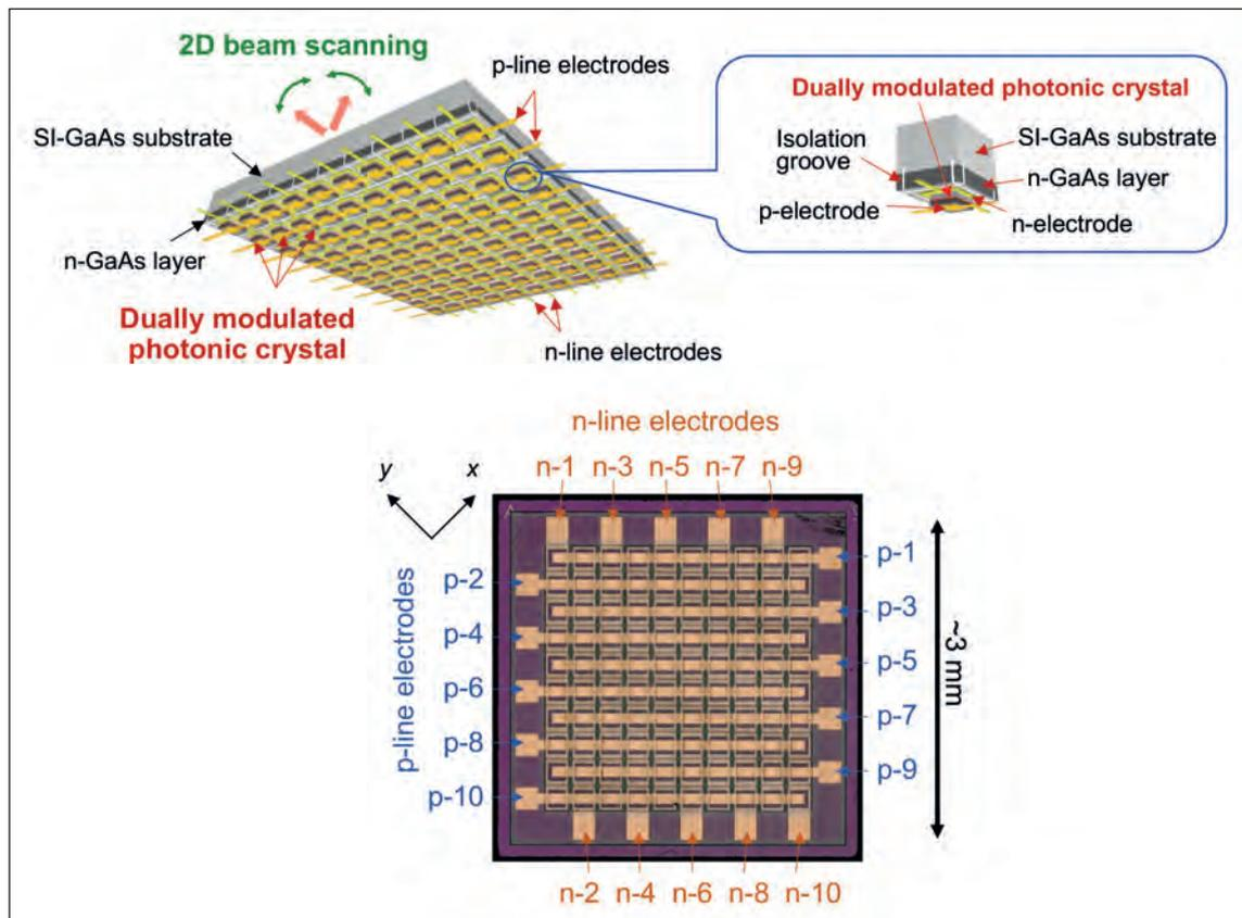
➤ Figure 12. On-chip array of dually modulated PCSELS for beam emission in various directions in two dimensions. (Top) schematic of the entire device. (Bottom) microscope image of the bottom of the chip.
