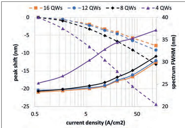
► Figure 3. Spectral parameters versus current density for green LEDs shown in Figure 2. Dashed lines indicate the full-width at half maximum (FWHM) and solid lines indicate the peak wavelength shift relative to its value at a low current density.
