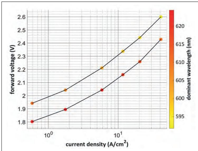
► Figure 7. Current density versus voltage (J-V) curves for two representative InGaN red LEDs with different wavelength targets. The colour bar indicates the dominant wavelength of the emission spectrum at each point.
