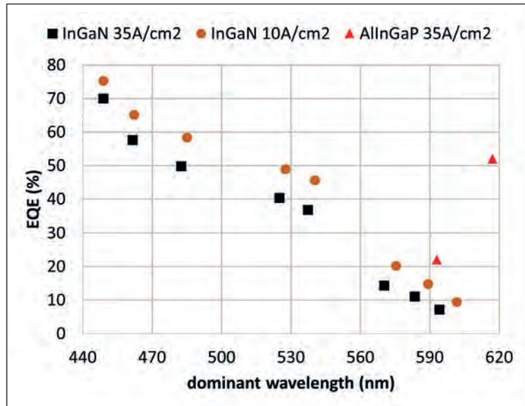
➤ Figure 1. The external quantum efficiency of state-of-the-art visible wavelength LEDs with 1 mm by 1 mm dimensions and a hemispherical dome encapsulation.
