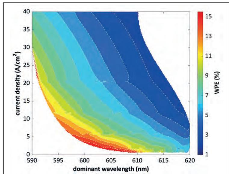
➤ Figure 6. Contour plot of the InGaN red wall-plug efficiency (WPE) as a function of current density and dominant wavelength at that current density. The plot is constructed from WPE and spectrum measurements versus current density for many encapsulated 1 mm by 1 mm LEDs of the same epitaxy design with varied quantum well indium concentrations.
