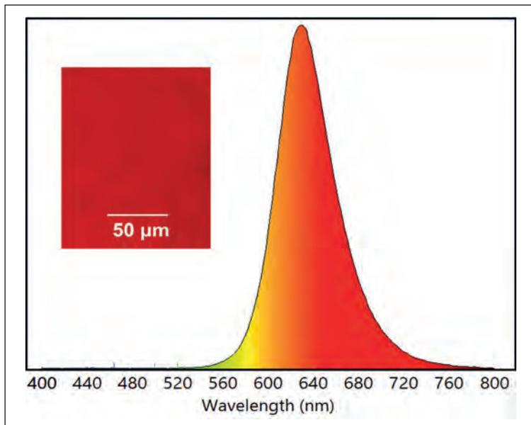
► Figure 4. Spectrum of an InGaN red LED operated at 40 A cm<sup>-2</sup> with a peak wavelength of 638 nm and a dominant wavelength of 610 nm. The inset shows the emitting surface observed under an optical microscope at the forward voltage of 1.8 V, corresponding to the onset of light emission.
