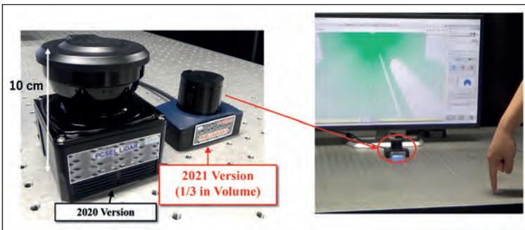
➤ Figure 9. Further miniaturization of a lidar system. The 2021 version is just one-third of the volume of its predecessor from 2020.
