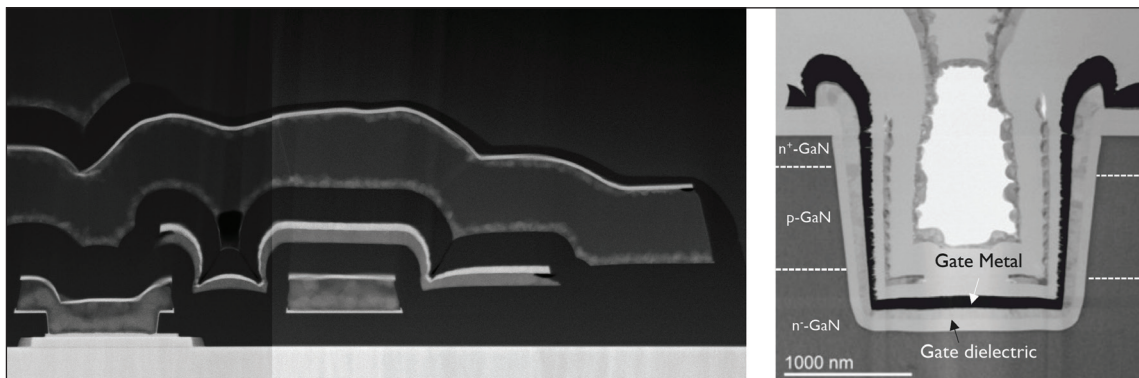
➤ Figure 1: Cross-section STEM of (a) the p -GaN gate architecture used in lateral devices and (b) the trench gate MOS architecture used in vertical devices.
