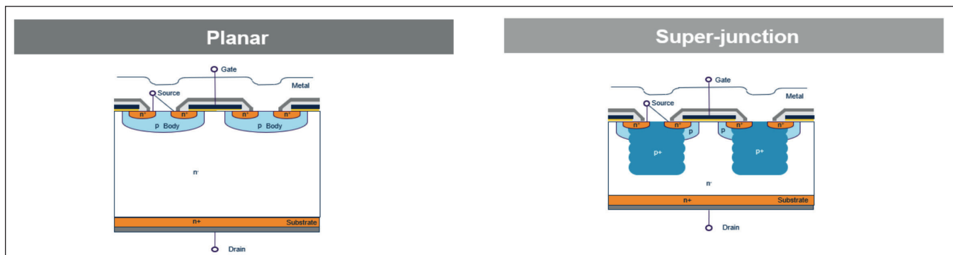
➤ Figure 3. High Voltage Silicon MOSFET technology evolution
