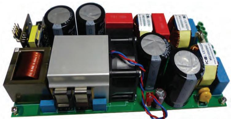
Figure 3: Infineon high efficiency, bi-directional, totem-pole PFC stage demonstrator, using SiC MOSFETs
