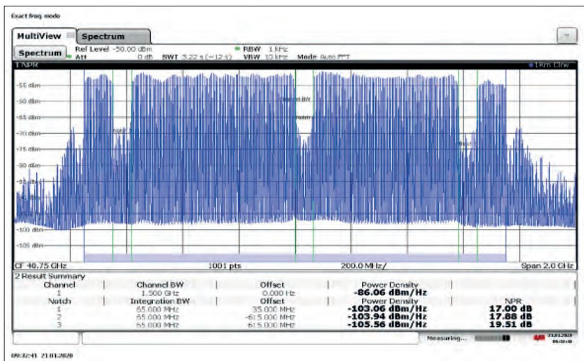
Figure 8. Measured noise-to-power (NPR) of the solid-state power amplifier (SSPA). This measurement was made by driving the SSPA with 301 uncorrelated carriers occupying a frequency band of 1.5 GHz large and applying three notches 65 MHz large.
