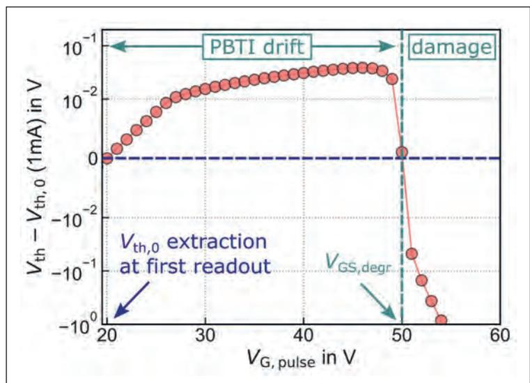
Figure 5. Infineon has developed a new form of stress test for SiC MOSFETs. A series of voltages are applied, each 1 V higher than the previous one, and the threshold voltage is recorded. As the stress voltage incrementally increases, initially the threshold voltage increases as well, due to a positive bias temperature instability. But beyond a certain value the threshold voltage plummets and the device is irreversibly damaged.
