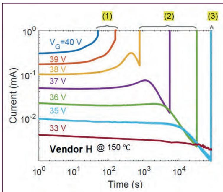
Figure 8. Researchers have identified three different regimes for SiC MOSFETs subjected to gate-stress tests. When the gate voltage is 39 V or more, the gate current accelerates; for voltages of 38 V to 35 V, initially the current varies, before a rapid hike; and for a voltages of 33 V, current falls steadily.
