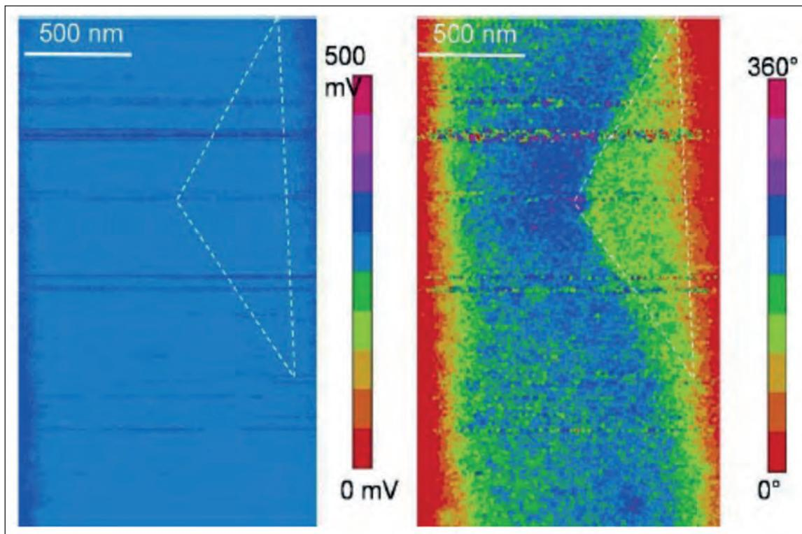
Figure 3. Investigations of threading dislocations by a partnership between CNR-IMM and STMicroelectronics have involved scanning capacitance microscopy measurements. A map of the amplitude of this signal (right) reveals a constant doping concentration; the phase of the signal (left) uncovers local variations in minority carrier concentration, and enables identification of a charge distribution associated with a triangular defect.
