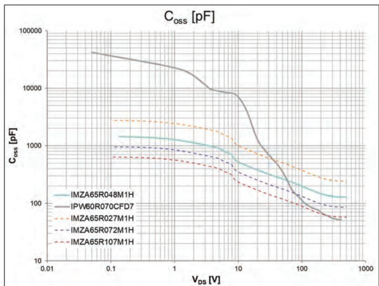
Figure 2: SiC device output capacitance varies far less with drain voltage than silicon
