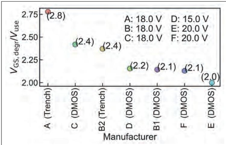
Figure 6. Research at Infineon has uncovered a difference in the failure rate reduction factor of two orders of magnitude between SiC MOSFETs made by different manufacturers. This implies that the most reliable devices have roughly one hundred times fewer failures in the field than the most unreliable devices.
