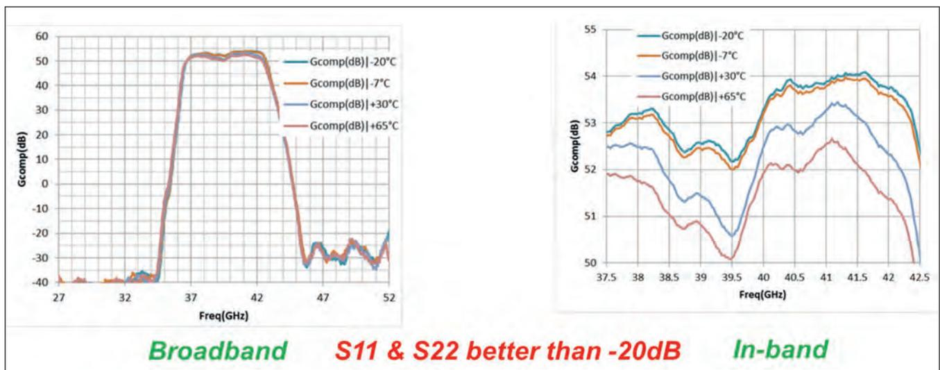
Figure 7. Measured large-signal performances of the solid-state power amplifier.
