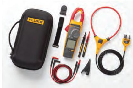
The Fluke 377 and 378 use FieldSense technology to sense voltage and current through the clamp jaw, with only a connection to earth needed for reference. With no direct connection with live components, the risk of electric shock and arc flash is minimized.
