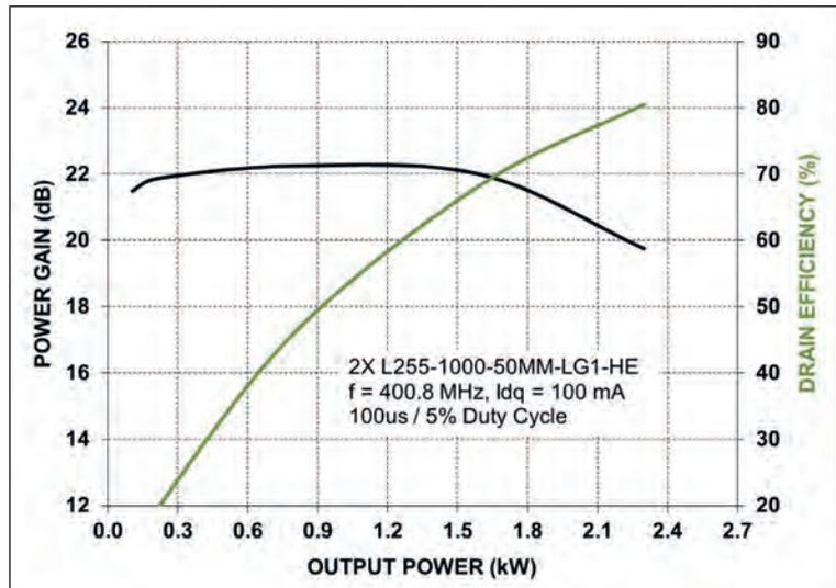
Figure 1. Measured RF power gain and drain efficiency versus output power at 145 V bias and 400.8 MHz. Quiescent current is 100 mA. 6  $\Omega$  series gate resistors help to stabilise the transistor with 20 dB gain at 2 dB compression and 2.3 kW saturated power. Drain efficiency peaks at 80 percent. In CW operation at 100 V bias, saturated power is 1.2 kW with the same 80 percent peak drain efficiency.
