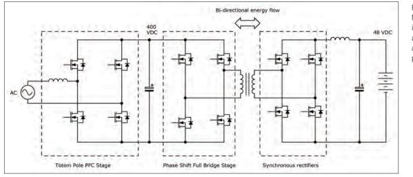
Figure 1: MOSFETs in bridge arrangements as a bi-directional power converter
