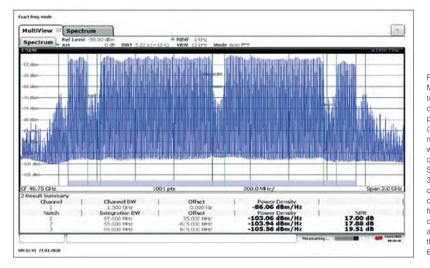
Figure 8. Measured noiseto-power (NPR) of the solid-state power amplifier (SSPA). This measurement was made by driving the SSPA with 301 uncorrelated carriers occupying a frequency band of 1.5 GHz large and applying three notches 65 MHz large.
