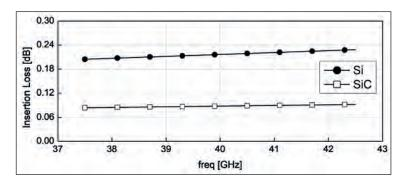
Figure 1. Simulated insertion loss of a transmission line with a  $Z_0 = 50 \ \Omega$  characteristic impedance and 1 mm length realized on silicon (filled symbols) and SiC (empty symbols) substrates.
