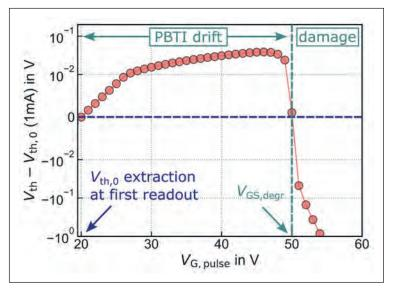
Figure 5. Infineon has developed a new form of stress test for SiC MOSFETs. A series of voltages are applied, each 1 V higher than the previous one, and the threshold voltage is recorded. As the stress voltage incrementally increases, initially the threshold voltage increases as well, due to a positive bias temperature instability. But beyond a certain value the threshold voltage plummets and the device is irreversibly damaged.
