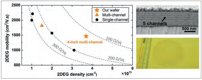
Figure 2 (left) 2DEG density versus 2DEG mobility for the single-channel and multi-channel AlGaN/GaN materials reported in the literature and measured on the wafer detailed in this article. (right) cross-sectional scanning electron microscopy image and top-view photo of the 4-inch, five-channel, GaN-on-sapphire wafer produced by Enkris Semiconductor Inc.
