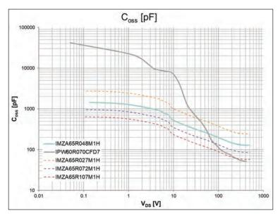
Figure 2: SiC device output capacitance varies far less with drain voltage than silicon
