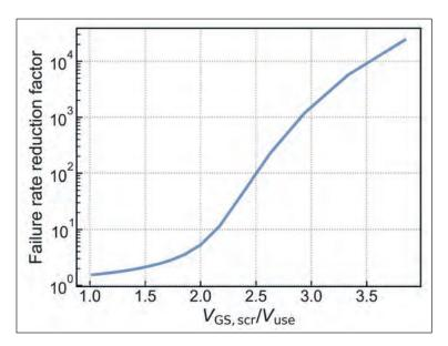
Figure 4. Engineers at Infineon have drawn on previous work (Aichinger and Schmidt, IRPS2020, 3B4\_042) that relates a failure rate reduction factor to the ratio of the screening voltage ( $V_{\rm GS,scr}$ ) to the recommended gate use voltage provided by a datasheet ( $V_{\rm use}$ ). Combining this relationship with rapid stress tests enabled a comparison of the reliability of SiC MOSFETs produced by various vendors.
