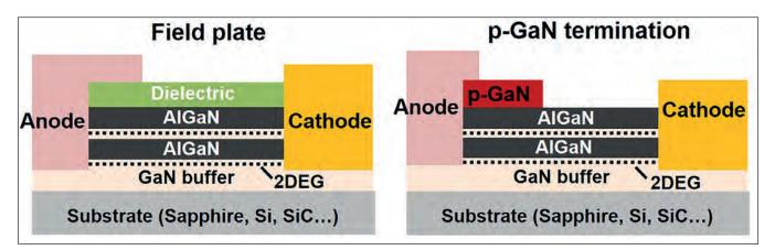
Figure 3. A conventional field plate termination (left) and Virginia Tech's novel *p*-GaN termination (right). Two channels are drawn to illustrate multi-channel structures.
