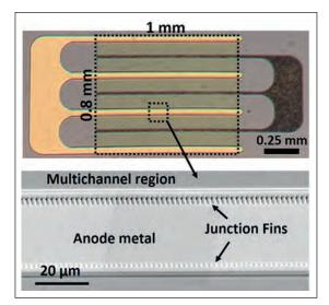
Figure 5 Top-view microscopic images of the fabricated 1.5 A, 5 kV GaN power Schottky rectifier.
