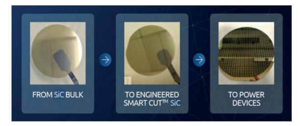
Figure 3. Pictures of bulk SiC (left), Smart Cut SiC (centre), and Smart Cut SiC with devices (right).
