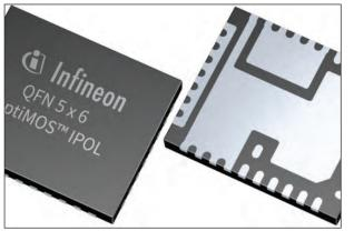
Infineon's TDA38740 and TDA38725 digital IPOL buck regulators support up to 40 A and 25 A output current, respectively and come with a PMBus interface.
