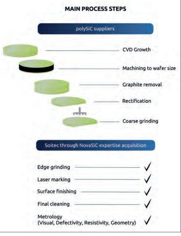
> Figure 3. Main process steps for manufacturing polycrystalline SiC.
