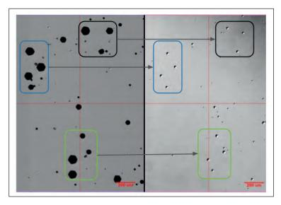
> Figure 4. Etching with potassium hydroxide enables crystal defect characterization. Decorations are easily visible with an optical microscope, allowing comparison between a single-crystal SiC donor (left) and SmartSiC (right).
