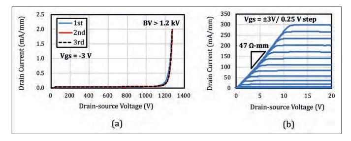
Figure 6. (a) Measured off-state breakdown of the fabricated hybrid HEMT. Repetitive current-voltage (I-V) sweep curves up to 2 mA/mm show high stability against avalanche current stress. (b) On-state characteristics. Owing to current flow via the low-resistance 2DEG, a low on-resistance of 47 Ω-mm and high saturation current of 300 mA/mm were measured.
