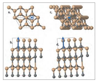
Figure 3. JMOL simulation of 4H-SiC lattice. Blue arrow shows the direction of c-axis of the crystal. (a) view through the channelling direction; (b) sideview; (c) tilted lattice; (d) tilted lattice sideview.
