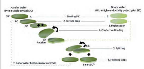
Figure 2. The unique, patented Smart Cut process of Soitec, adapted to SiC material.
