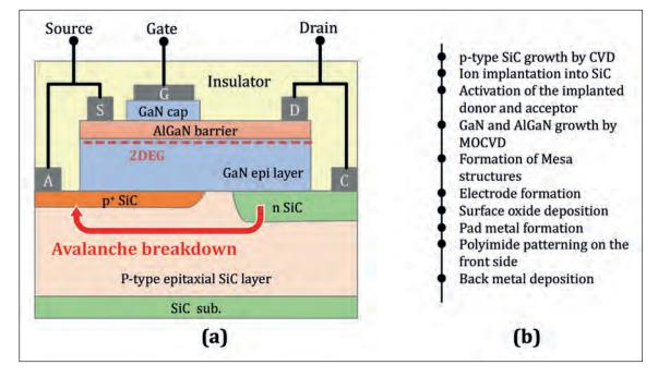
GaN and SiC. This novel transistor, which solves the issue of destructive breakdown, features a SiC-based anti-parallel p-n diode, monolithically integrated to a GaN HEMT (see Figure 5(a)) for a diagram of this device, and Figure 3(c) for the equivalent circuit). This hybrid device has five electrodes: the source, gate and drain of the GaN HEMT structure; and the anode and cathode of the SiC diode structure.
