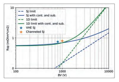
> Figure 8. Trade-off curves of breakdown voltage and on-state resistance for unipolar and superjunction devices with experimental data shown
