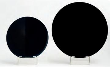
> Figure 6. SmartSiC wafers in 150 mm and 200 mm formats.
