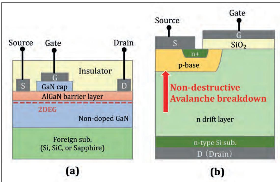
➤ Figure 2. (a) Schematic cross-section of a conventional GaN HEMT and a (b) silicon D MOSFET.
