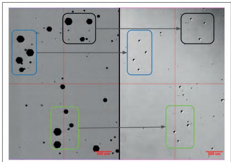
➤ Figure 4. Etching with potassium hydroxide enables crystal defect characterization. Decorations are easily visible with an optical microscope, allowing comparison between a single-crystal SiC donor (left) and SmartSiC (right).
