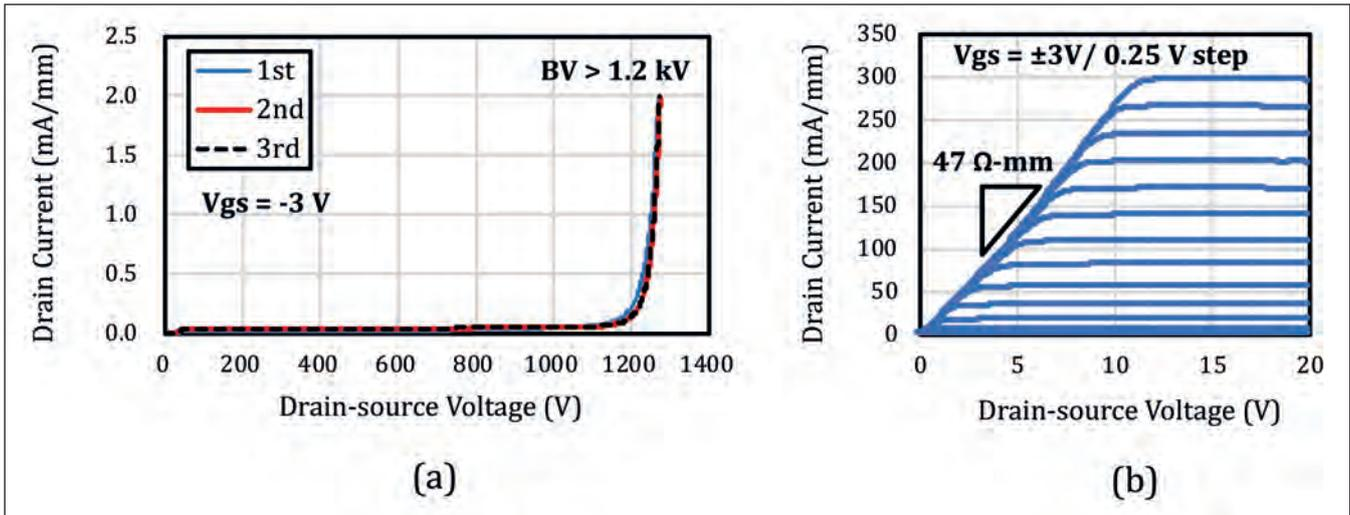
► Figure 6. (a) Measured off-state breakdown of the fabricated hybrid HEMT. Repetitive current-voltage (I-V) sweep curves up to 2 mA/mm show high stability against avalanche current stress. (b) On-state characteristics. Owing to current flow via the low-resistance 2DEG, a low on-resistance of 47 Ω-mm and high saturation current of 300 mA/mm were measured.
