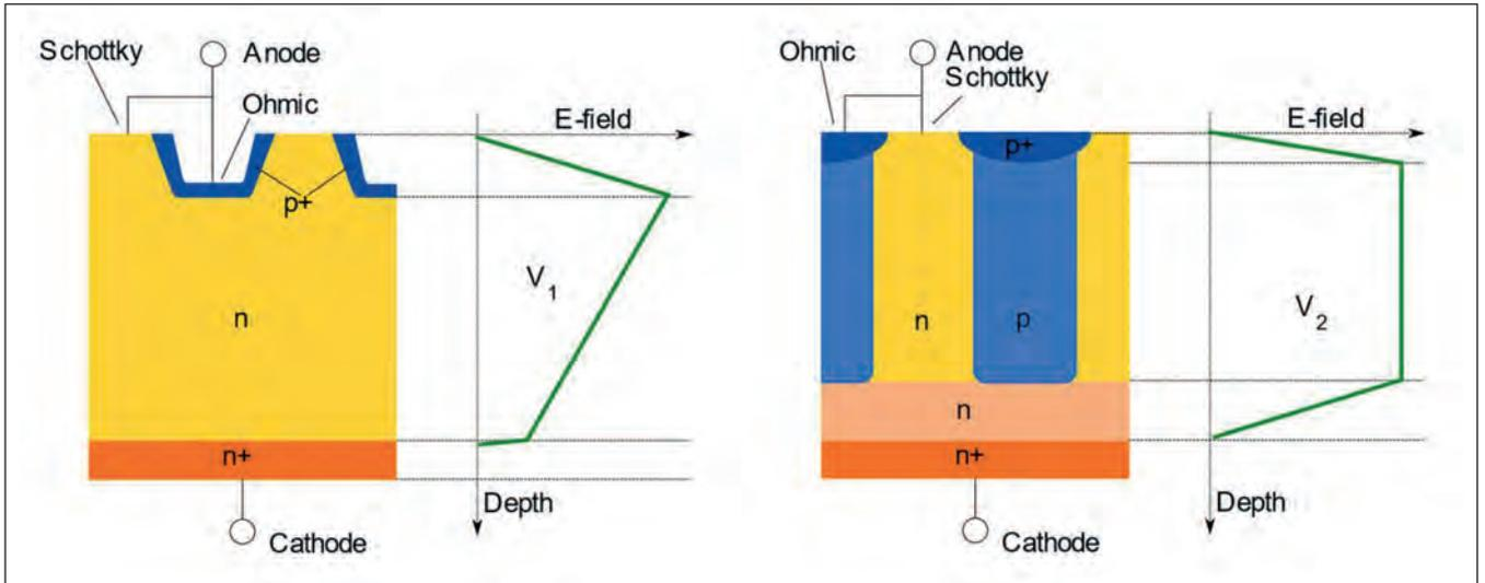
► Figure 2. Schematic diagram of JBS diode with unipolar drift region (left) and superjunction JBS diode (right).
