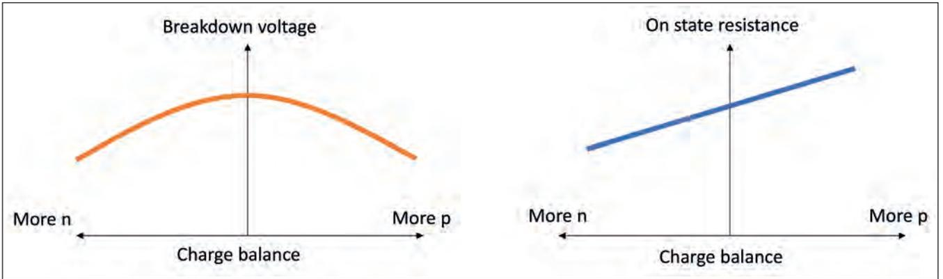
➤ Figure 6. Predicted behaviour of the superjunction device.
