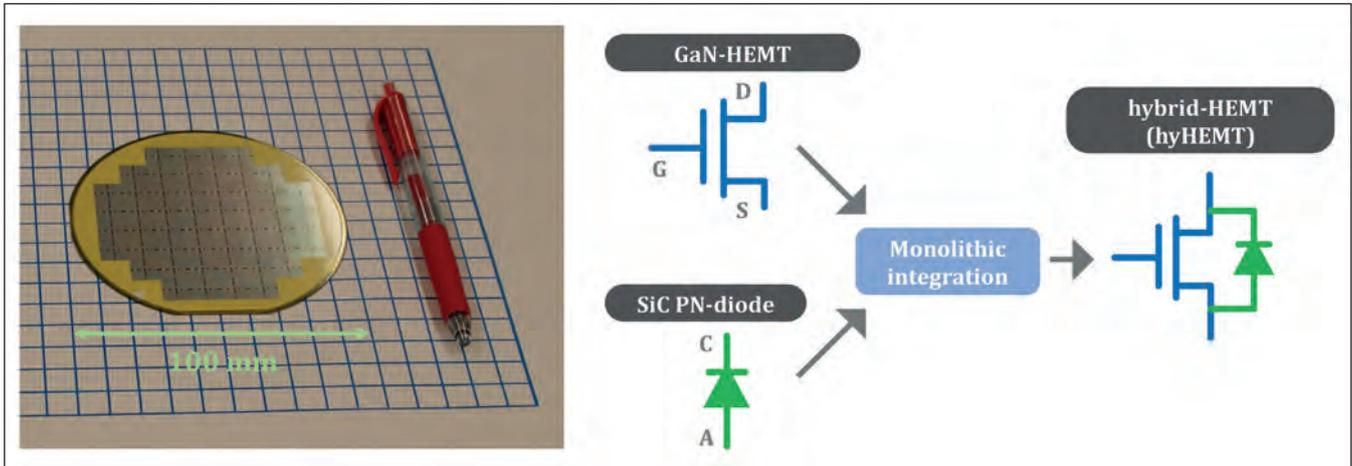
➤ Figure 1. Photograph of fabricated hybrid HEMTs on a 100 mm SiC substrate (left) and an equivalent circuit (right).
