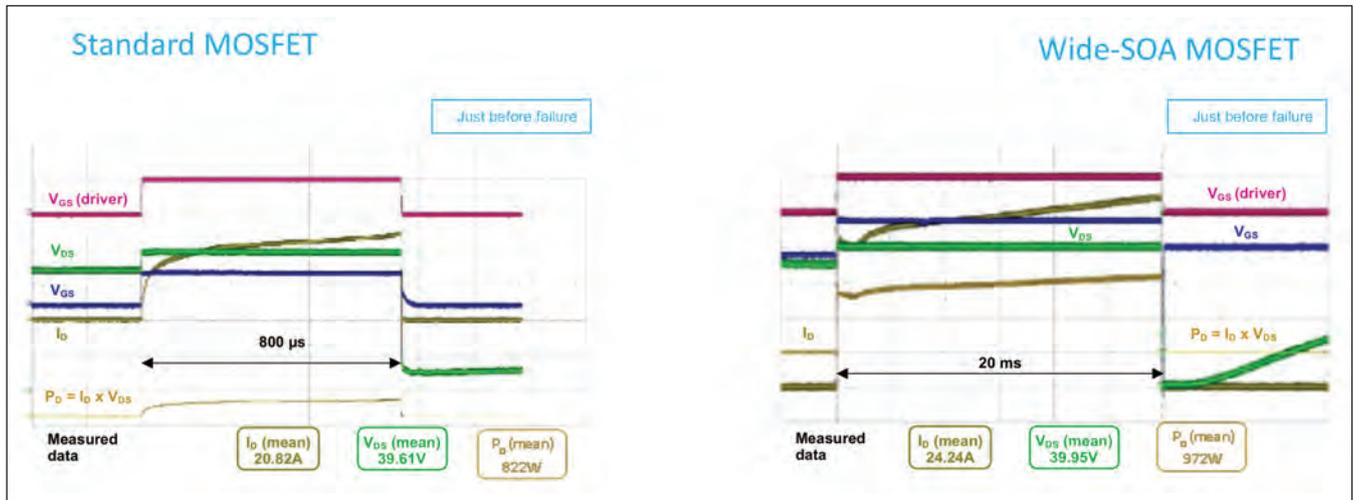
➤ Fig. 6. Measured waveforms for standard trench MOSFET and wide-SOA device at a fixed drain current.
