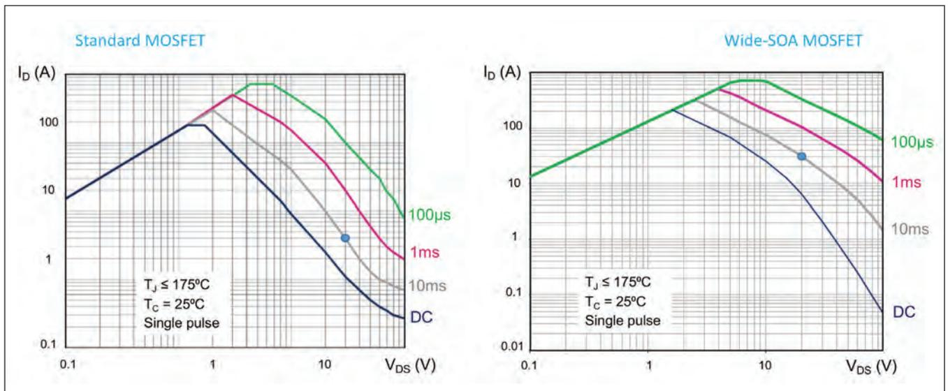
➤ Fig. 4. SOA diagram for the standard trench MOSFET and wide-SOA device.
