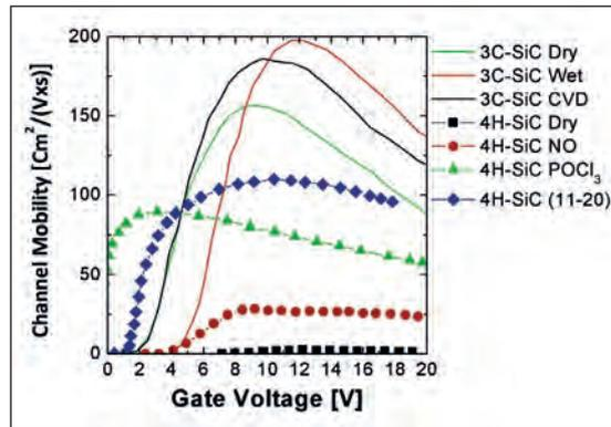
► Figure 1. Comparison between the channel mobility in 3C-SiC and 4H-SiC.
