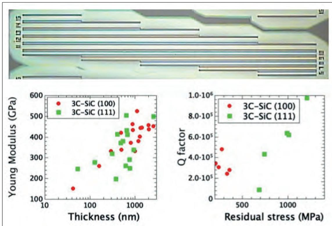
➤ Figure 5. (up) Double clamp beam array with different lengths and widths. (left) An increase in the Young's modulus with increasing thickness is observed in both (100) and (111) 3C-SiC. (right) The Q-factor increase at high residual stress is essentially in (111) 3C-SiC. In (100) 3C-SiC, the residual stress is lower, as is the Q-factor.
