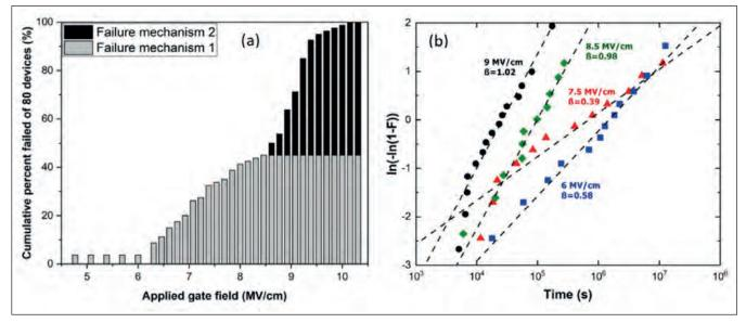
▶ Figure 4: Distribution of failures of 3C-SiC MOS capacitors for varying electric fields (a) and corresponding Weibull distributions (b), taken from F. Li *et al.* Materials **14** (2021). The time dependent dielectric breakdown analysis is conducted at electric field values of 6 - 9 MV cm<sup>-1</sup>. The failure percentage increases steadily up to an electric field strength of 8.5 MV cm<sup>-1</sup>, above which, the failure number rapidly increases to 100 percent.
