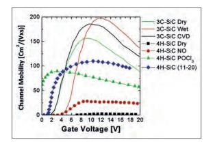
► Figure 1. Comparison between the channel mobility in 3C-SiC and 4H-SiC.
