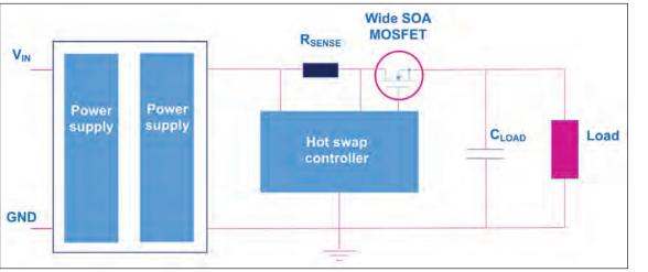
➤ Fig. 1. Hot swap system block diagram.
