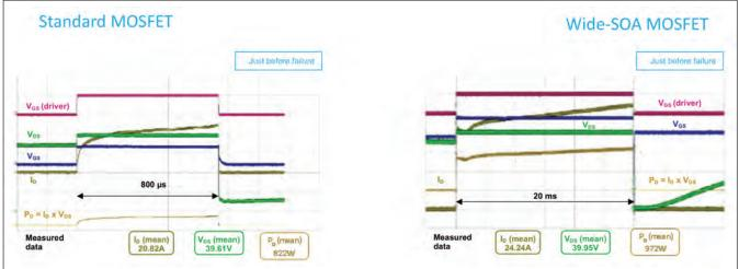
Fig. 6. Measured waveforms for standard trench MOSFET and wide-SOA device at a fixed drain current. value of on-resistance  $R_{\rm DS(on)}$ . Moreover, the high values of the  $V_{\rm GS}$  voltage are fixed in order to be higher than the ZTC point of the power MOSFET, which therefore does not present any thermal drift issue.
