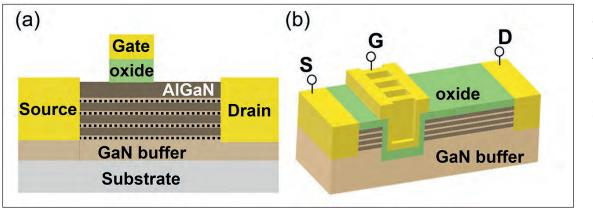
Figure 1. The multichannel AlGaN/GaN HEMT with a planar gate (a) and a trigate architecture (b).
