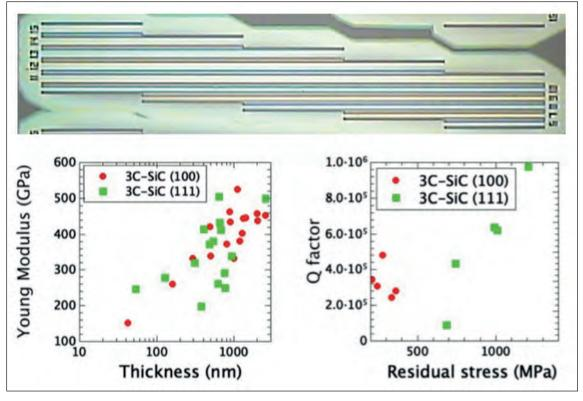
> Figure 5. (up) Double clamp beam array with different lengths and widths. (left) An increase in the Young's modulus with increasing thickness is observed in both (100) and (111) 3C-SiC. (right) The Q-factor increase at high residual stress is essentially in (111) 3C-SiC. In (100) 3C-SiC, the residual stress is lower, as is the Q-factor.
