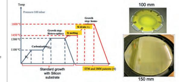
schematics of the CVD process for the bulk growth of 3C-SiC. 100 mm and a 150 mm wafers are reported too.
