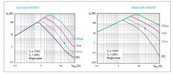
> Fig. 4. SOA diagram for the standard trench MOSFET and wide-SOA device.
