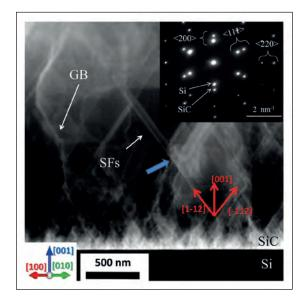
and stacking faults in the epilayer, and voids in silicon beneath the hetero-interface (see Figure 2). These defects are device killers. However, their threat can be diminished by growing several tens of microns of 3C-SiC. This relatively thick film reduces their density, with some defects totally annihilated. Note that the defect density and the surface morphology strongly depend on the orientation of the silicon substrate.
