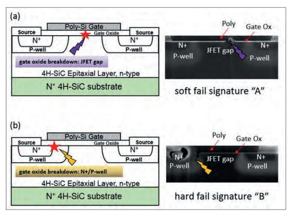
Figure 4. Schematic cross section as well as focused ion beam, cross-sectioned scanning electron microscopy images, showing gate oxide rupture after negative gate bias time-dependent dielectric breakdown (TDDB): (a) in the JFET gap for the type 'A' soft-fail electrical signature, (b) the n<sup>+</sup>/p<sup>-</sup> well for the type 'B' hard-fail electrical signature. Adapted from S. Ganguly et al., IEEE International Reliability Physics Symposium (IRPS), pp. 8B.1-1-8B.1-6, 2022.
