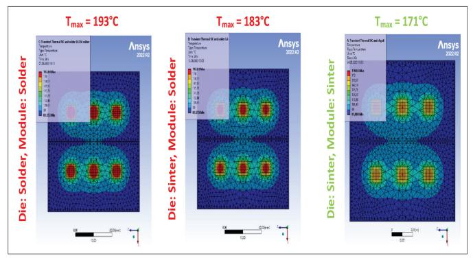
Figure 2: ANSYS simulation results of the steady-state temperature distribution of various packaging concepts. From left to right: Module and die soldered, module soldered and die sintered, fully sintered module. Simulation details: PLoss = 202 W per chip, SiC die size 5x5x0.15mm<sup>3</sup>.
