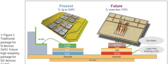
Figure 1 (right side) shows an advanced packaging concept optimized to achieve highest reliability
