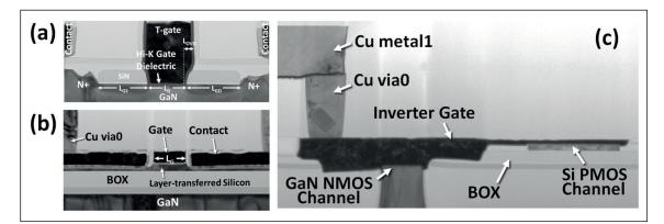
as necessitating additional fabrication steps and masks, these intra-connects added path resistance when accessing the underlying GaN transistors. In contrast, our latest process for producing GaN and silicon CMOS transistors leads to a shared backend copper interconnect stack, eliminating the need for additional intra-connects and masks.
