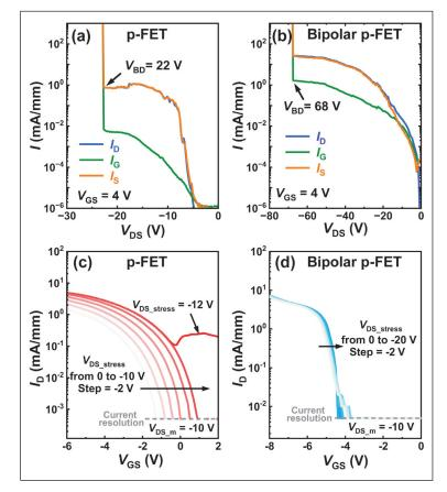
> Figure 4. (a) Off-state leakage current and breakdown characteristics of (a) the conventional p-FET and (b) bipolar p-FET. Plots of pulsed drain current as a function of gate-source voltage ( $I_p$ - $V_{GS}$ ) of (c) the p-FET and (d) the BiPFET measured with various drain-source stress voltages ( $V_{DS \ stress}$ ).
