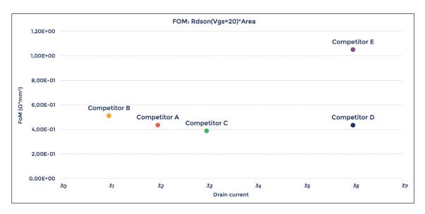
> Performance comparison of discrete SiC MOSFETs figure of merit.
