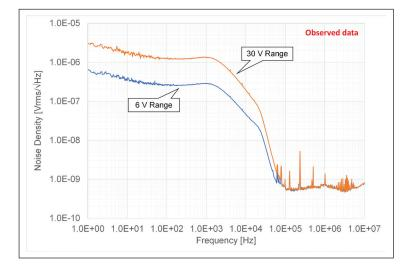
Figure 4. Voltage source noise density with the combination of a source metre and a low-noise filer adapter. The qubit's sensitivity to noise necessitates continual monitoring of the potential noise source. Figure 2 illustrates how this effect becomes more pronounced when extending the cables because the DC power supply rack is at a distance from the entrance of the cryostat or if the power supply is in the lower sections of the rack.
