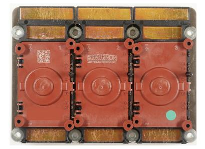
Analized Semikron - Danfoss Empack 1200V SiC module optical view from above.
