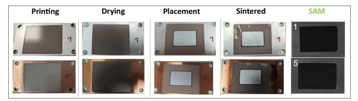
> Figure 5: Process flow and scanning acoustic microscopy (SAM) images of PE360P sintered AMBs substrates on Ag plated and bare Cu baseplates.
