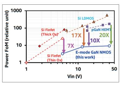
▶ Figure 2. Benchmarking the power figure-of-merit ( $R_{ON}xQ_{GG}$ ) of the GaN transistor of this work shows: a performance that's around a 20-fold better than the *p*GaN HEMT and around a 30-fold better than silicon LDMOS at 40 V; a 10-17-fold better performance than silicon LDMOS and a *p*GaN HEMT at 12-15 V, and 7-fold better performance than a silicon finFET at 5 V.
