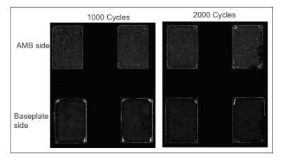
Figure 6: SAM images of the AMB side and the baseplate side after thermal cycling. The area of each of the substrates is approximately 1000 mm<sup>2</sup>. TCT condition: -55°C/+150°C (20min dwell time).
