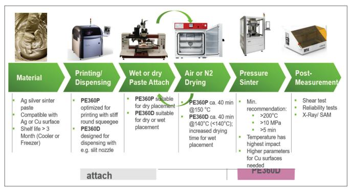
> Figure 4: Process flow for both PE360 variants, including wet or dry placement. PE360P is designed for printing applications such as stencil or screen printing and ensures a processability of more than 8h on the printing machine. PE360P was designed for placement of molded packages or bare substrates in the range of 40x40 mm<sup>2</sup> up to 100x100 mm<sup>2</sup> onto the pre-dried paste.
