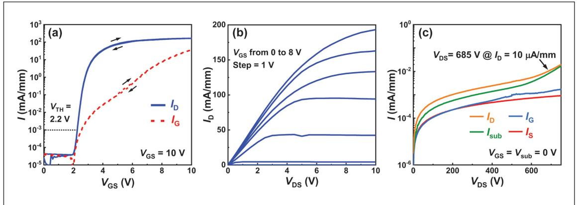
a value comparable to that of conventional  $p$ -GaN gate HEMTs (see Figure 5(a) and (b)). This robust conduction capability indicates that the 2DEG channel is not significantly impacted by regrowth of the  $n$ - $p$ - $n$  stack.
