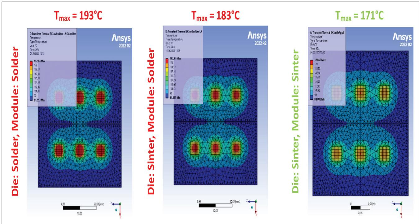
➤ Figure 2: ANSYS simulation results of the steady-state temperature distribution of various packaging concepts. From left to right: Module and die soldered, module soldered and die sintered, fully sintered module. Simulation details: PLoss = 202 W per chip, SiC die size 5x5x0.15mm<sup>3</sup>.
