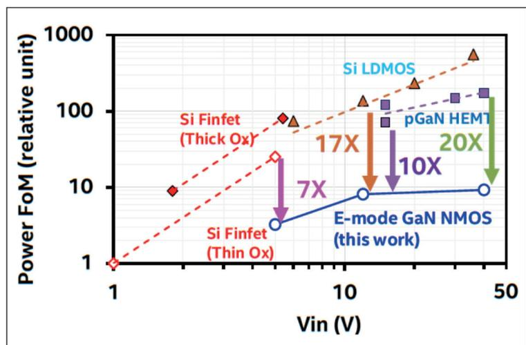
► Figure 2. Benchmarking the power figure-of-merit ( $R_{ON} \times Q_{GC}$ ) of the GaN transistor of this work shows: a performance that’s around a 20-fold better than the pGaN HEMT and around a 30-fold better than silicon LDMOS at 40 V; a 10-17-fold better performance than silicon LDMOS and a pGaN HEMT at 12-15 V, and 7-fold better performance than a silicon finFET at 5 V.
