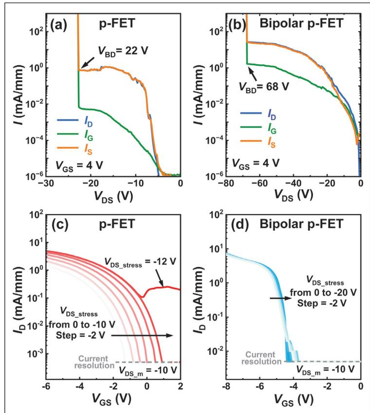
➤ Figure 4. (a) Off-state leakage current and breakdown characteristics of (a) the conventional  $p$ -FET and (b) bipolar  $p$ -FET. Plots of pulsed drain current as a function of gate-source voltage ( $I_D$ - $V_{GS}$ ) of (c) the  $p$ -FET and (d) the BiPFET measured with various drain-source stress voltages ( $V_{DS\_stress}$ ).
