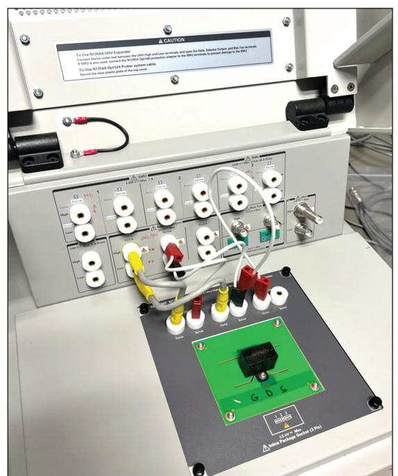
➤ Test setup for the SiC discrete MOSFETs.
