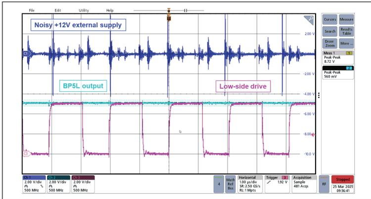
➤ Figure 8. An LDO cleaning up the ripple voltage from the external supply.
