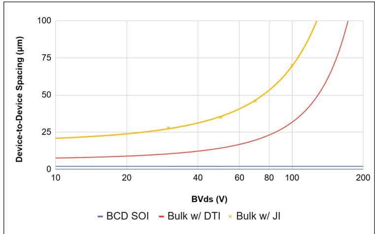
➤ Fig 7. Device-to-device isolation spacing based on BCD with Power-SOI and DTI, BCD with bulk and DTI and BCD with bulk and junction isolation [3]
