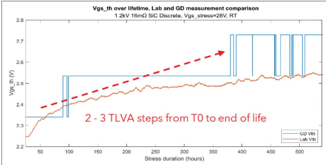
➤ Figure 2. Vth Drift Over Time As Measured by GD3162 (Courtesy to NXP Semiconductors)
