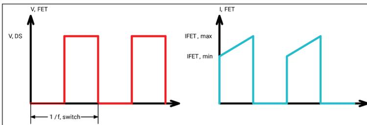
➤ Figure 12. High-side voltage and current stresses in a synchronous buck converter.
