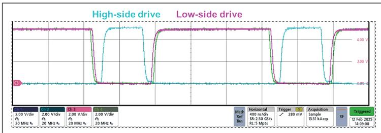
➤ Figure 10: Extending the dead time ensures that the opposite gate drive has reached 0V.
