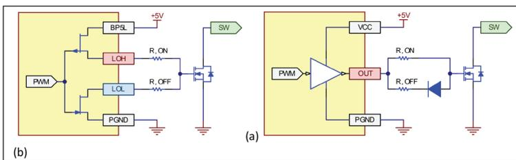
➤ Figure 11. A split-gate output gate driver (a) does not require an additional diode compared to totem-pole (b) output.
