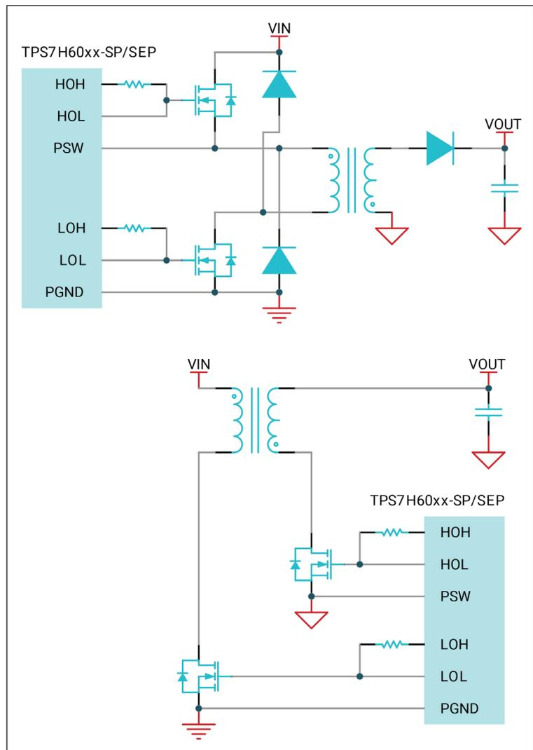
➤ Figure 7. Isolating the high-side gate driver can enable the use of higher-efficiency topologies.
