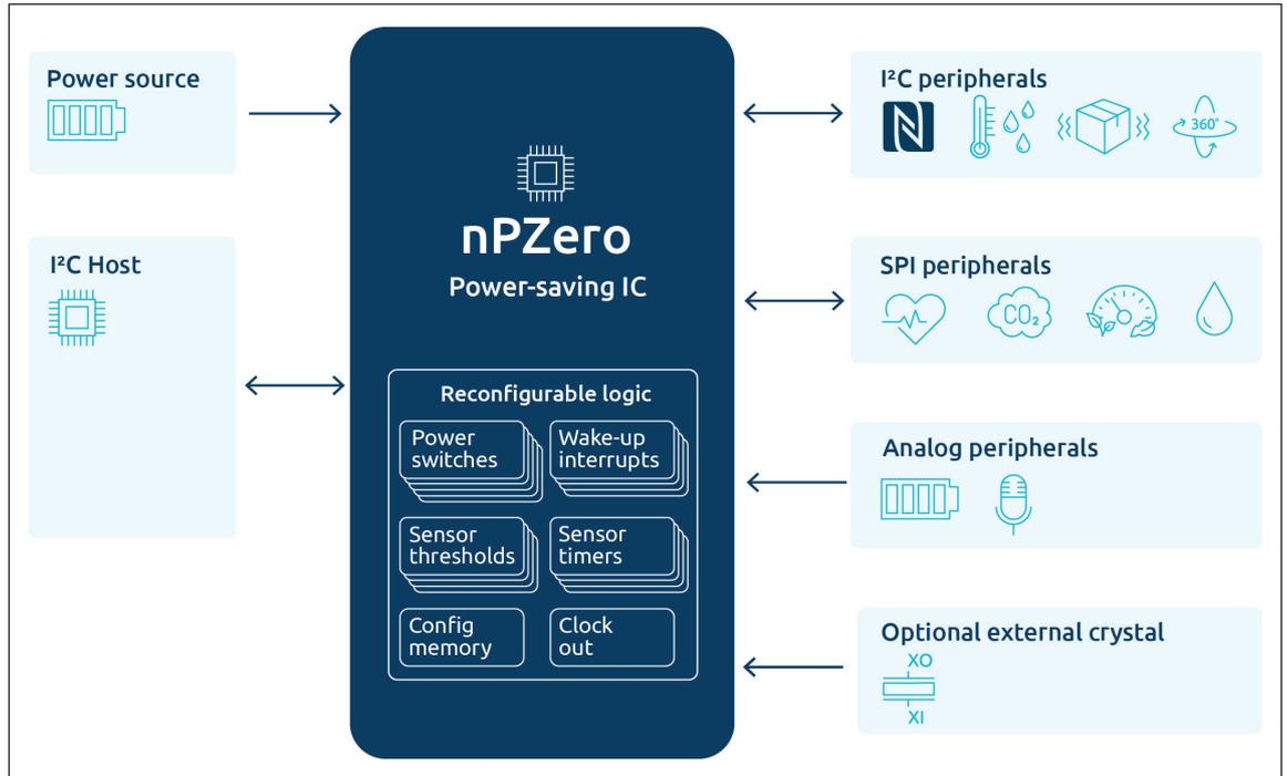
and manually edited in the tool if needed. Additionally, the tool can analyse the state of power switches and serial interfaces in a running system, allowing the user to evaluate the efficiency of a given implementation, and tune the configuration of the nPZero device to their requirements. Hardware implementation is also straightforward: the nPZero requires only a few external passive components, and an optional crystal for more accurate time keeping.
