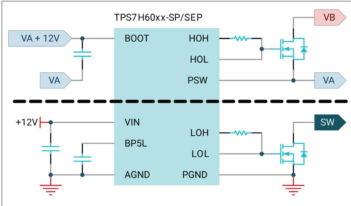
➤ Figure 6. The high-side gate driver in functionally isolated applications.
