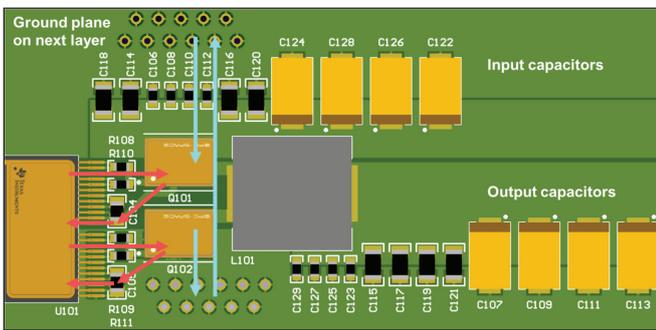
➤ Figure 15. Increasing the gate-drive path to enable better input-capacitor placement.
