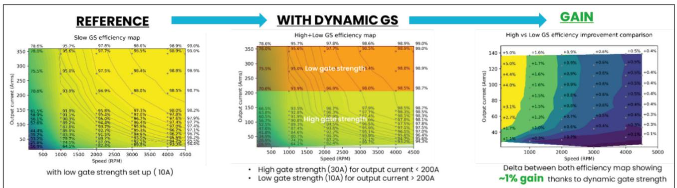
➤ Figure. 1 GD3162 Efficiency Gain with Dynamics GS (Courtesy to NXP Semiconductors)
