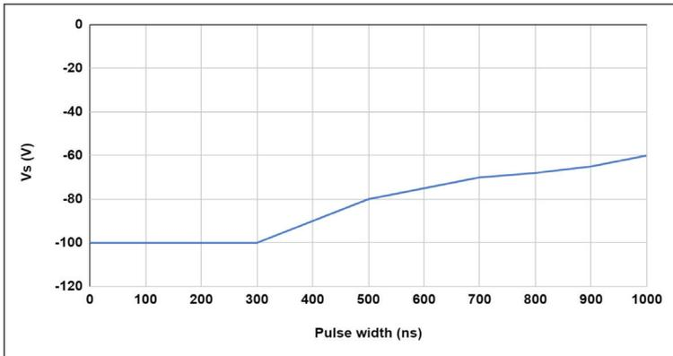
➤ Figure 5. Example of NTSOA of an Auto Power-SOI based gate driver IC [2]
