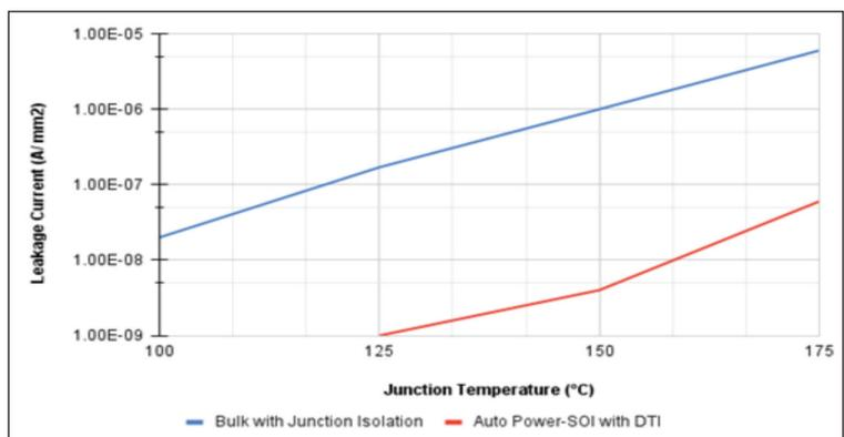
➤ Fig 8. Comparison of leakage currents for Power-SOI with DTI and bulk substrate with junction isolation [4]
