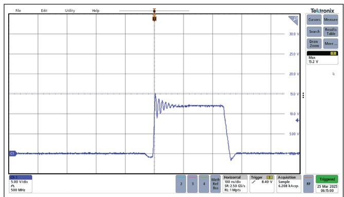
➤ Figure 16. Reduced ringing time and total voltage stress on the switch node.
