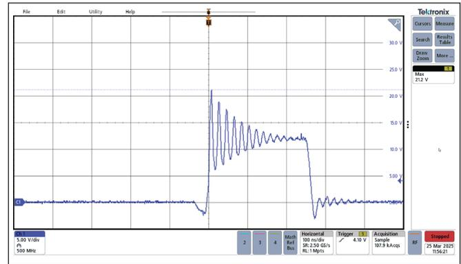
➤ Figure 14. Large switch-node ringing on a synchronous buck-converter design.
