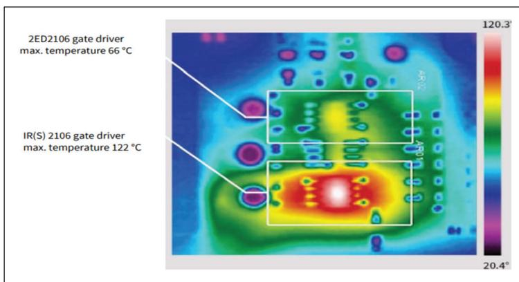
➤ Figure 6. Example of the comparison of Auto Power-SOI based gate driver IC and bulk based gate driver IC [2]
