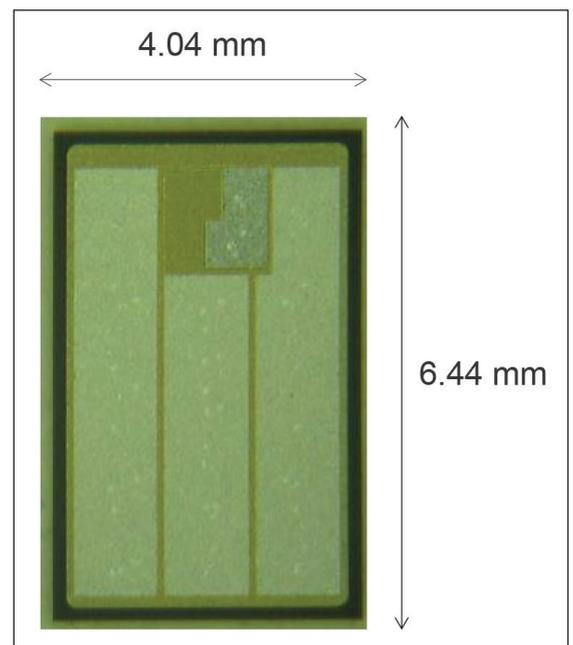
➤ Figure 1. Example bare chip (courtesy of Wolfspeed)
