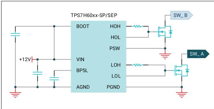
► Figure 4. Using the half-bridge device as a dual low-side gate driver simplifies connections.
