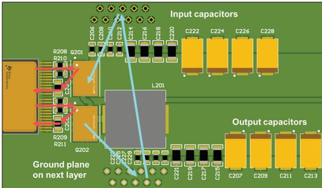
➤ Figure 13. A buck converter PCB design with a minimized gate path.
