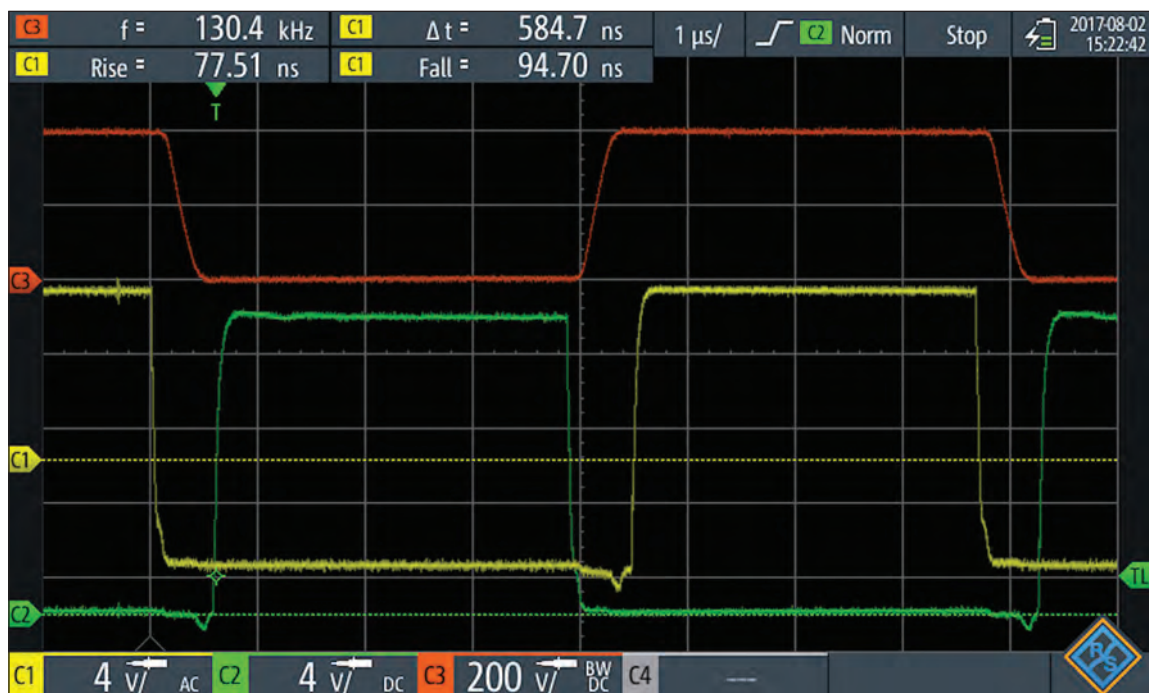
Figure 1: Measuring the gate source (C1, C2) and output voltage (C3) of a resonant converter; all figures and graphic representations in this article are courtesy of Rohde & Schwarz (R&S)
