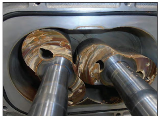
Figure 3 Vibration signal from a pump on an atomic layer deposition tool (left) and a photo of material deposited on internal components.
