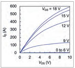
Figure 8. I<sub>D</sub>-V<sub>DS</sub> characteristics  $(V_{GS} = 0 - 18 V)$ at  $T_i = 25 \,^{\circ}\text{C}$ The VMOSFETs exhibit a high current capability of 200 A DC and 600 A pulse.
