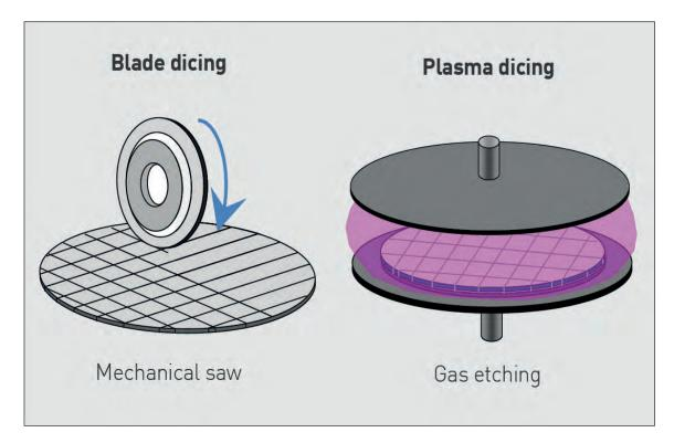
Figure 1: Blade dicing & Plasma dicing processing
