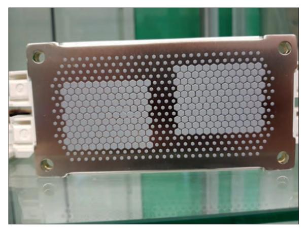
Figure 3: Base plate bottom surface with TIM applied
