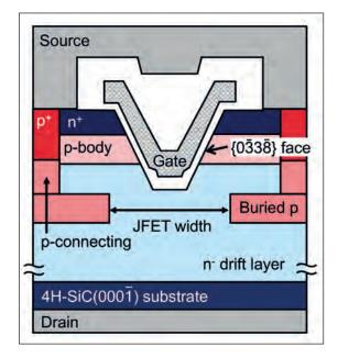
directed at high power conversion efficiency, so that the devices can handle hundreds of amps and have a breakdown voltage above 1 kV. These transistors feature 4H-SiC{0338} trench side walls that have a higher channel mobility than other SiC crystal faces (see Figure 3 for a diagram of this structure). Using this design, channel resistance can be reduced while realising a high channel density.
