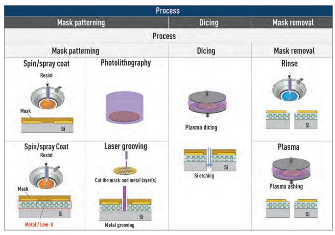
Figure 2: Panasonic's chemical etch dicing process
