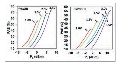
Figure 7. High power-added efficiencies are demonstrated with supply voltages from 3.5 V to as low as 1 V. Efficient PA operation well below 2 V surpasses the minimum cut-off supply voltage achievable by typical GaAs HBTs and highlights the potential of Intel's high-  $\!\kappa$  GaN transistor to extend battery life, and to realise efficient envelope-tracking RF PA.
