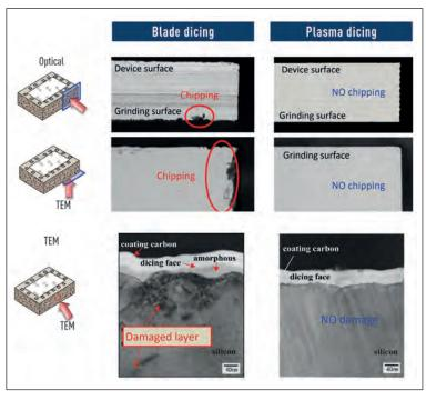
Figure 3: Damage evident on chip samples using blade dicing (left); none present when plasma dicing is used
