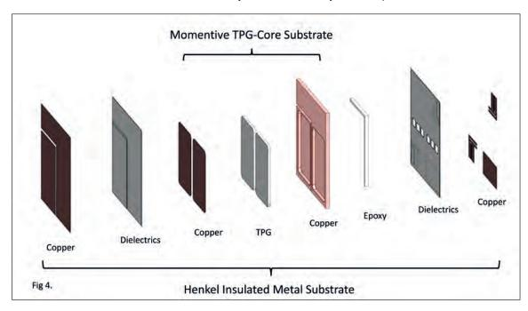
Figure 4. A seven-layer thermal pyrolytic graphite-core insulated metal substrate structure utilising proprietary materials and processing technologies from Momentive Quartz Technologies and Henkel.
