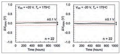
Figure 11. Stable threshold voltage of a VMOSFET under a high temperature gate bias test of  $V_{GS} = +20 \text{ V}$  (left) and -20 V (right) at  $T_a = 175 \,^{\circ}\text{C}$ .
