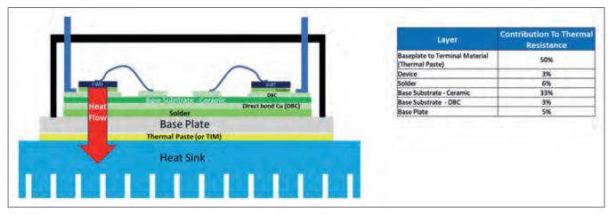
Figure 1: Heat flow pathway through module and layer contributions
