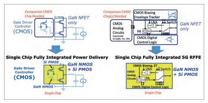
Figure 9. Single-chip fully integrated power delivery and RF front-end units can be realised with Intel's three-dimensional monolithically integrated silicon PMOS stacked on GaN NMOS transistor technology.
