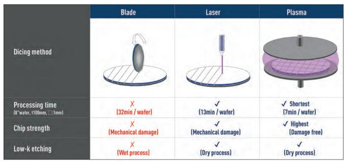
Figure 9: Summarises the different dicing processes and the advantages of the plasma dicing process
