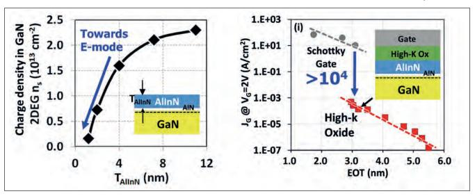
Figure 4. A high- $\kappa$  gate dielectric reduces gate leakage by more than four orders of magnitude at scaled equivalent oxide thickness (EOT) for higher performance.
