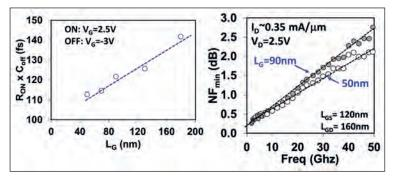
Figure 8. The excellent switch figure-of-merit,  $R_{ON} \times C_{OFF}$  and noise performance, NF $_{\min}$ , of the high- $\kappa$  e-mode GaN NMOS.
