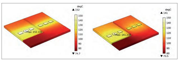
Figure 8. Thermal analysis of a SiC module using insulated metal substrates with a copper-core (left) and thermal pyrolytic graphite core (right). The results demonstrate the improvement in heat spreading by the two thermal pyrolytic graphite cores. More details are given in https://www. energy.gov/sites/prod/files/2019/06/f63/elt208 gurpinar 2019 o 4.9 3-41t.pdf
