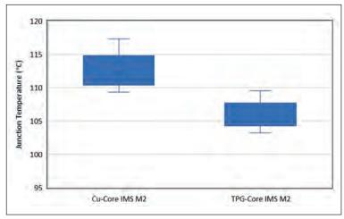
Figure 9. Plotting the SiC MOSFET junction temperature during power cycling revealed a 1.8 °C reduction in temperature range using the thermal pyrolytic graphite-core insulated metal substrate.
