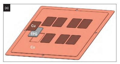
Figure 3. A substrate panel containing 8 thermal pyrolytic graphite (TPG) inserts (a); scanning electron microscope cross-section view of the TPG-core substrate (b), revealing a well aligned graphene stack and hermetic bonding; top-view of a thermal pyrolytic graphite-core substrate using ultrasound c-scan (c), showing a good bonding interface with little voiding
