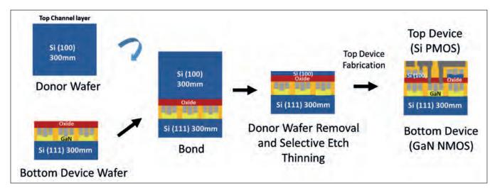
Figure 10. Intel's monolithic three-dimensional layer transfer process flow involves the transfer of a layer of single crystalline silicon from a 300 mm silicon (100) donor wafer onto a completed 300 mm GaN-on-silicon (111) wafer, prior to fabrication of the top silicon PMOS transistors.
