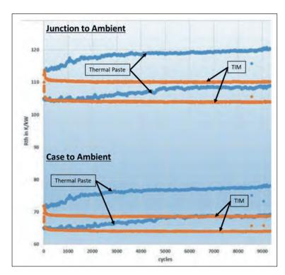
interface while dramatically reducing material pumpout. The use of the TIM improves the thermal transfer between power module and heat sink when compared to conventional heat conductive pastes, improving the long-term reliability and performance of the module. The TIM option will be available for LoPak modules beginning in June 2020.
