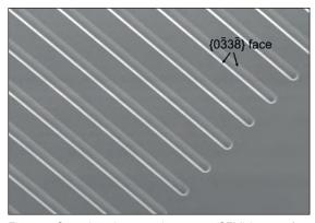
Figure 5. Scanning electron microscopy (SEM) image of a V-groove.
