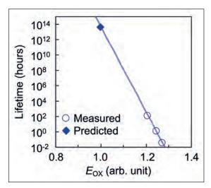
Figure 7. Long-term lifetime of VMOSFETs. Lifetime is estimated under a drain bias condition at T<sub>a</sub> = 175 °C in the case of a 10 percent cumulative failure rate. The predicted lifetime is equal to 200 years under a 0.1 ppm cumulative failure-rate condition.
