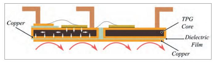
Figure 7. Conceptual module design using thermal pyrolytic graphite core to channel the waste heat away from the dies. More details are given in https://www.energy.gov/sites/prod/files/2019/06/f63/elt208\_gurpinar\_2019\_o\_4.9\_3-41t.pdf
