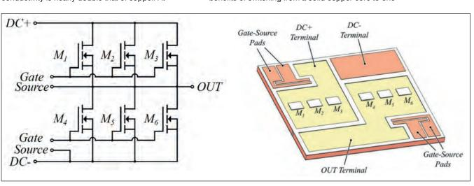
Figure 6. Electrical schematic of a half-bridge module (left) and insulated metal substrate circuit layout (right). More details are given in https:// doi.org/10.1115/IPACK2019-6436
