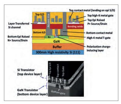
Figure 2. Intel has produced the first GaN transistors on a 300 mm silicon (111) wafer in one of its leading CMOS fabs. Its researchers have employed a new technique of three-dimensional monolithic integration by layer transfer to stack silicon PMOS transistors on top of GaN NMOS transistors to enable CMOS functionalities, for the first time in industry.
