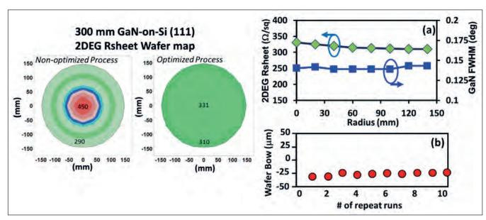
Figure 3. Optimised and uniform data from a manufacturable 300 mm GaN epitaxy process at Intel. Data distributions shown include: two-dimensional electron gas sheet resistance; GaN crystal quality, evaluated in terms of the the x-ray diffraction peak's full width at half-maximum (FWHM); and 300 mm wafer bow.
