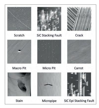
of 6" SiC pre- and post-grind wafers offering high precision frontside to back side correlation and die inking for process-induced killer defects on both sides of the wafer.
