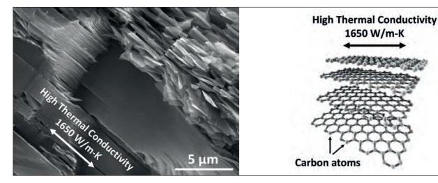
Figure 2. Cross-sectional view, provided by a scanning electron microscope, of Momentive Quartz Technologies' thermal pyrolytic graphite cores (left). An illustration of this material, showing well-aligned graphene basal planes (right).
