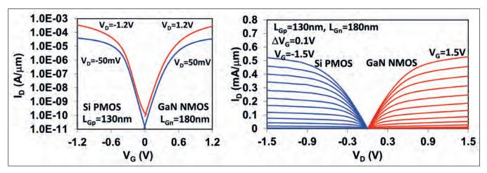
Figure 12. Current-voltage characteristics of the top layer channel length (LG is 130 nm) silicon PMOS transistor and the bottom channel length (L<sub>G</sub> 180 nm) GaN NMOS transistors. Dimensions have been chosen independently, to match drive current strengths and off-state leakages.
