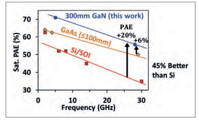
Figure 6. Intel's high-κ e-mode GaN NMOS transistor significantly outperforms GaAs and silicon/SOI across a frequency range spanning 1 GHz to 30 GHz.
