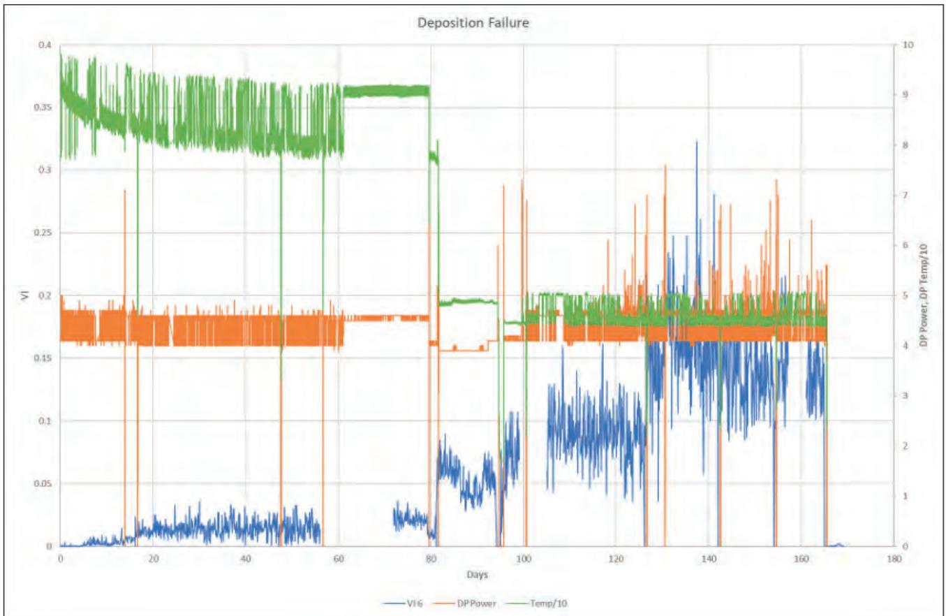
Figure 4: Dry pump power (orange) and temperature (green), and vibration data (blue) taken from a pump supporting an LP-CVD Si<sub>3</sub>N<sub>4</sub> batch deposition process
