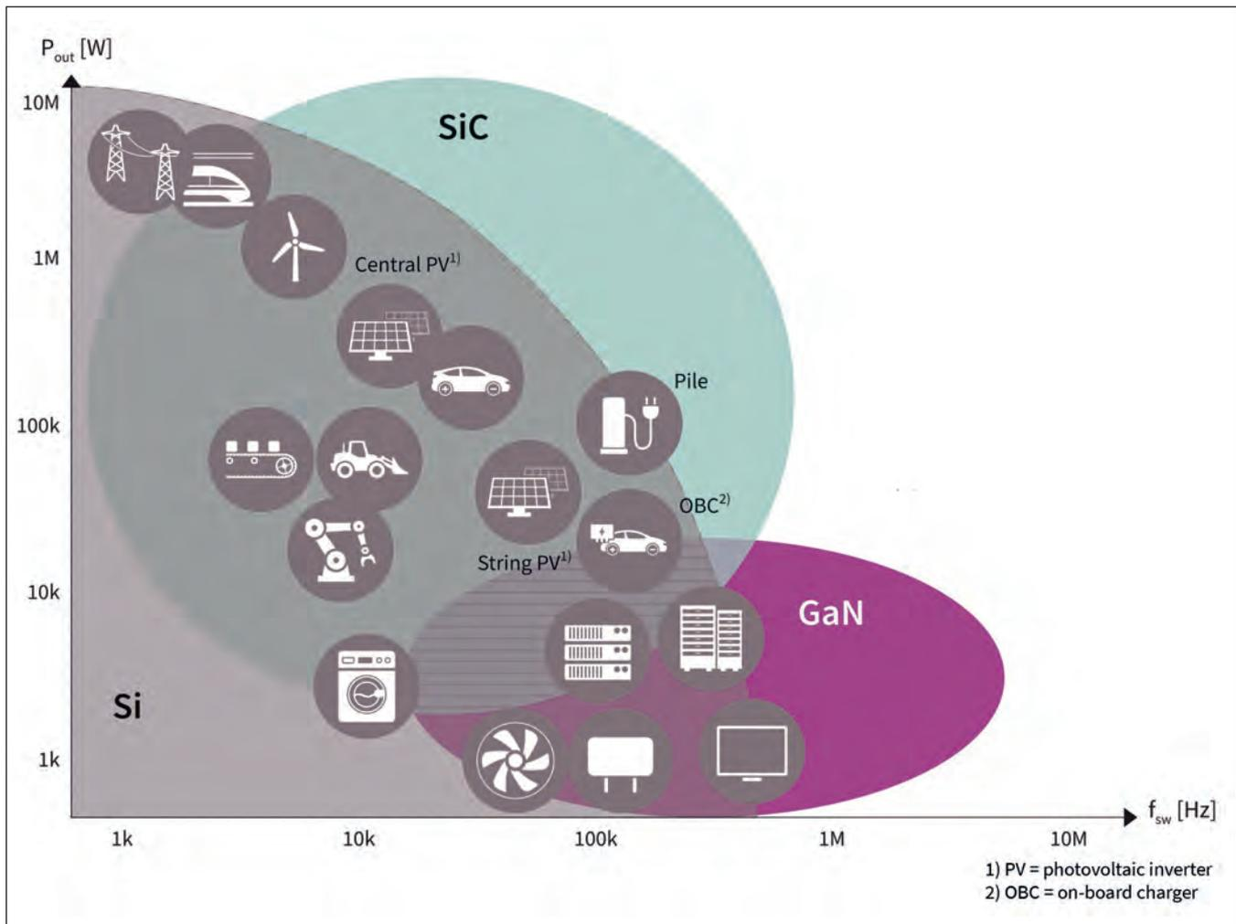
Figure 1: Mainstream silicon, complemented by SiC and GaN, delivers increased efficiency and a higher power density.
