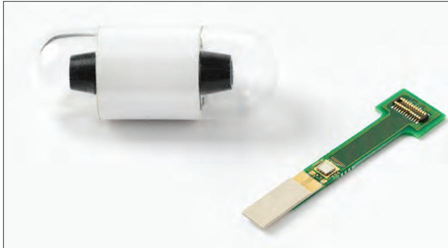
Mock-up of an ingestible pill (left) with prototype transceiver (right). The small rectangular chip is imec's ultra-small 400MHz radio (including antenna) for communication with the ingestible. It is pictured here on a green test board.
