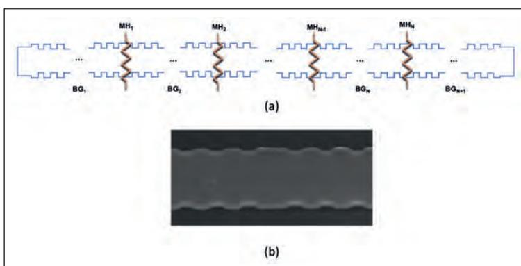
Figure 1. (a): Schematic top view layout of a Nth-order DFBR filter realized with a sidewall corrugated strip waveguide (b): Scanning electron microscope image of a fabricated grating. The devices were fabricated at the Inphotech Foundation facilities and at the James Watt Nanofabrication Centre at Glasgow University through the CORNERSTONE project.
