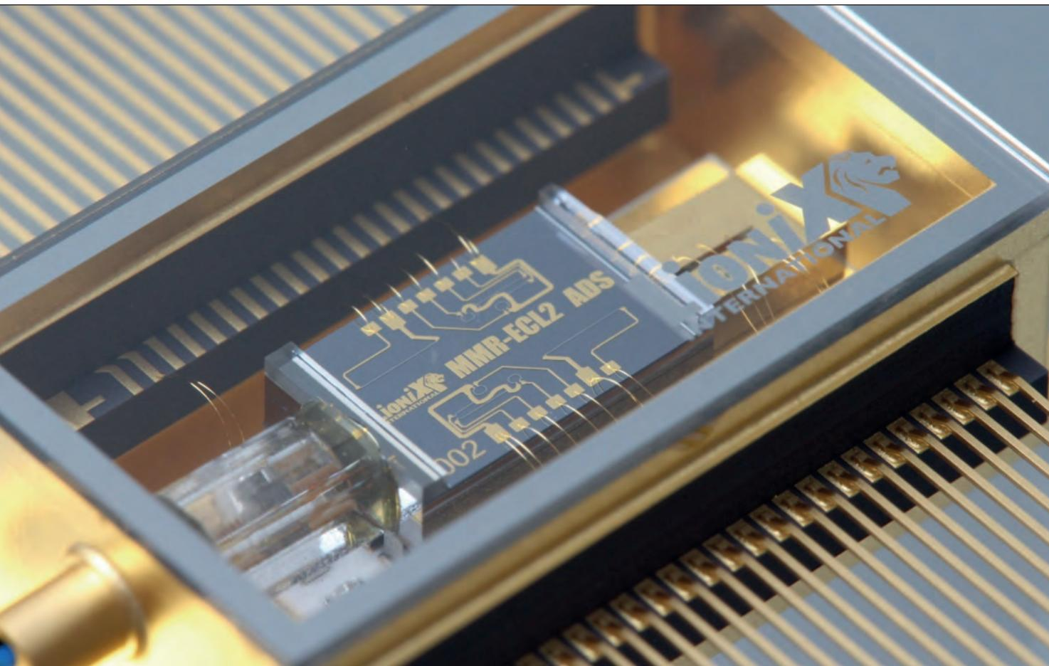
Figure 2. Narrow linewidth tunable laser based on hybrid assembly of an InP gain section and a tunable mirror made in TriPleX.
