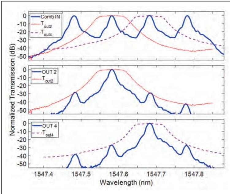
Figure 6. Spectral traces from two output ports of the demultiplexer when the DFBR filters are tuned to extract two adjacent tones from the input OFC (blue solid trace). Spectral transmissions of the corresponding DFBRs are also shown (dotted traces).
