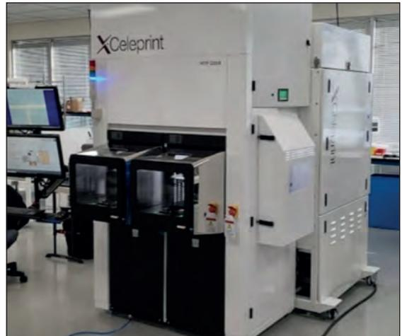
Figure 7: Automated MTP X-Celeprint tool capable of up to 200 mm wafer diameter fabrication.
