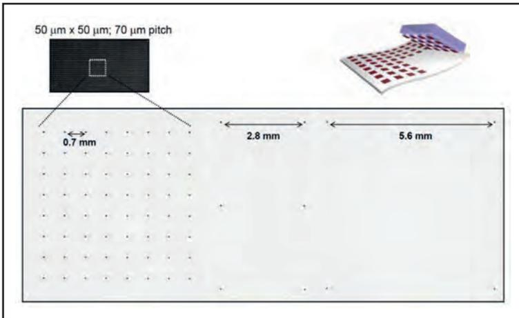
Figure 5: Example of fan-out capability for LEDs printed from a dense 70 micrometer source wafer (upper left) to a more sparsely populated target wafer of 0.7, 2.8, and 5.6 mm pitch (bottom). Adapted from Park et al. 3
