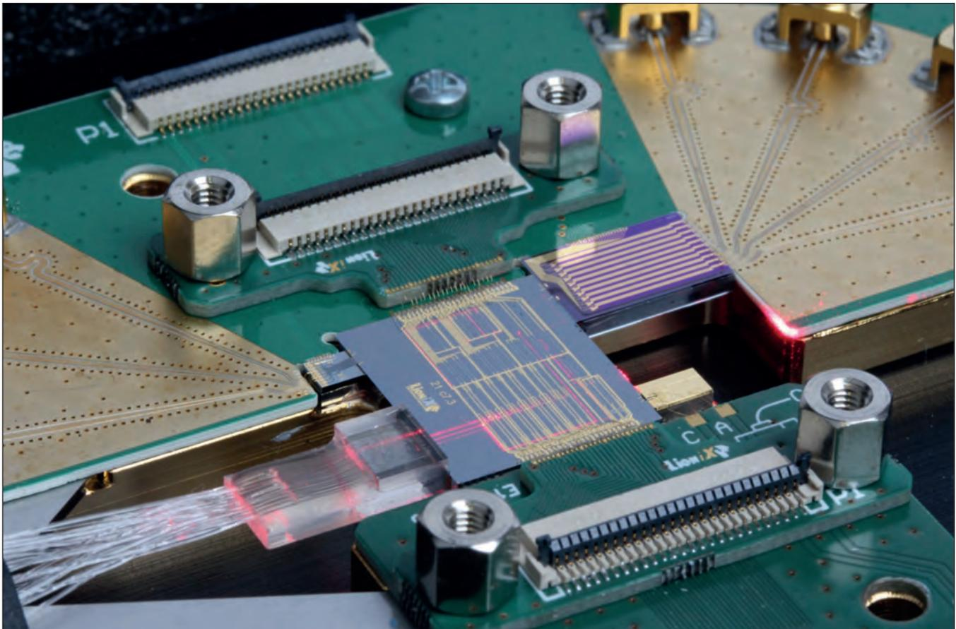
Figure 3. A RF-in/RF-out beamformer utilizing hybrid assembly to combine TriPleX true time delays and an InP laser, modulator and detectors.
