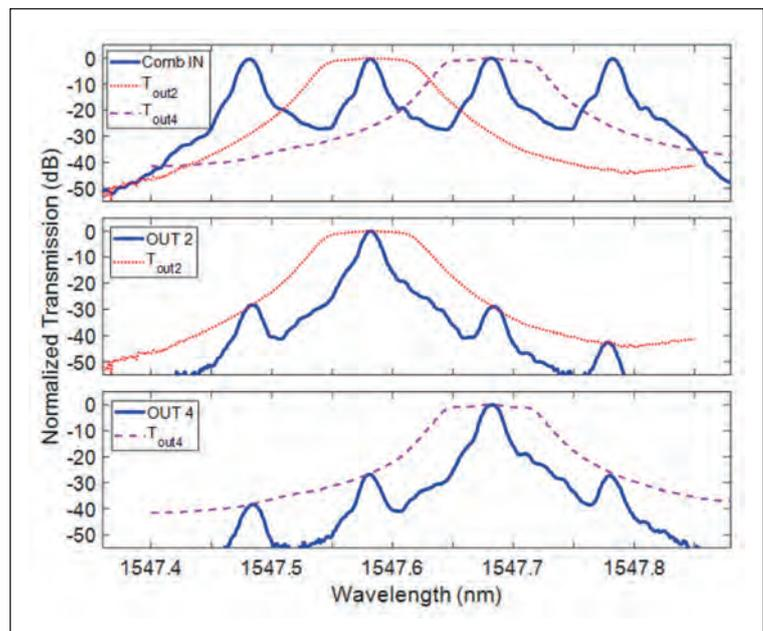
Figure 5. Normalized spectral transmission at the four output ports of the OFC demultiplexer when three DFBRs out of four are tuned through MHs for optimized response.
