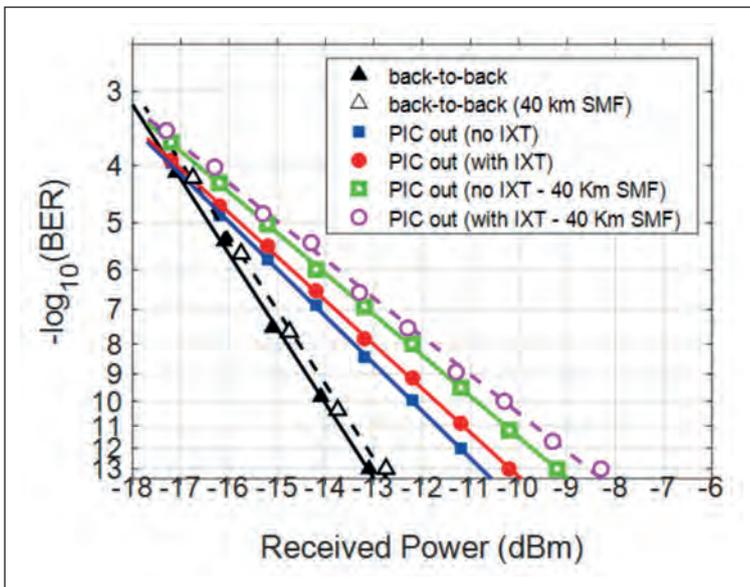
Figure 7. Results of BER measurements using the demultiplexed OFC tones for transmitting 12.5 Gbps-modulated on-off keying signals and evaluating the residual inter-channel crosstalk (IXT).
