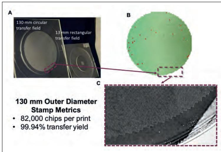
Figure 4: A) A PDMS stamp of a 130 mm circular (left) and 13 mm rectangular (right) transfer field. The 130 mm circular transfer field, matches a 150 mm wafer less a 10 mm edge, B) shows the device yield where pixels indicate successful prints and red pixels indicate failed prints. For 82,000 chips per print, 99.94% were successfully transferred. C) shows a close-up of the 130 mm circular transfer field at edge where the upper left portion is filled with PDMS stamp posts.
