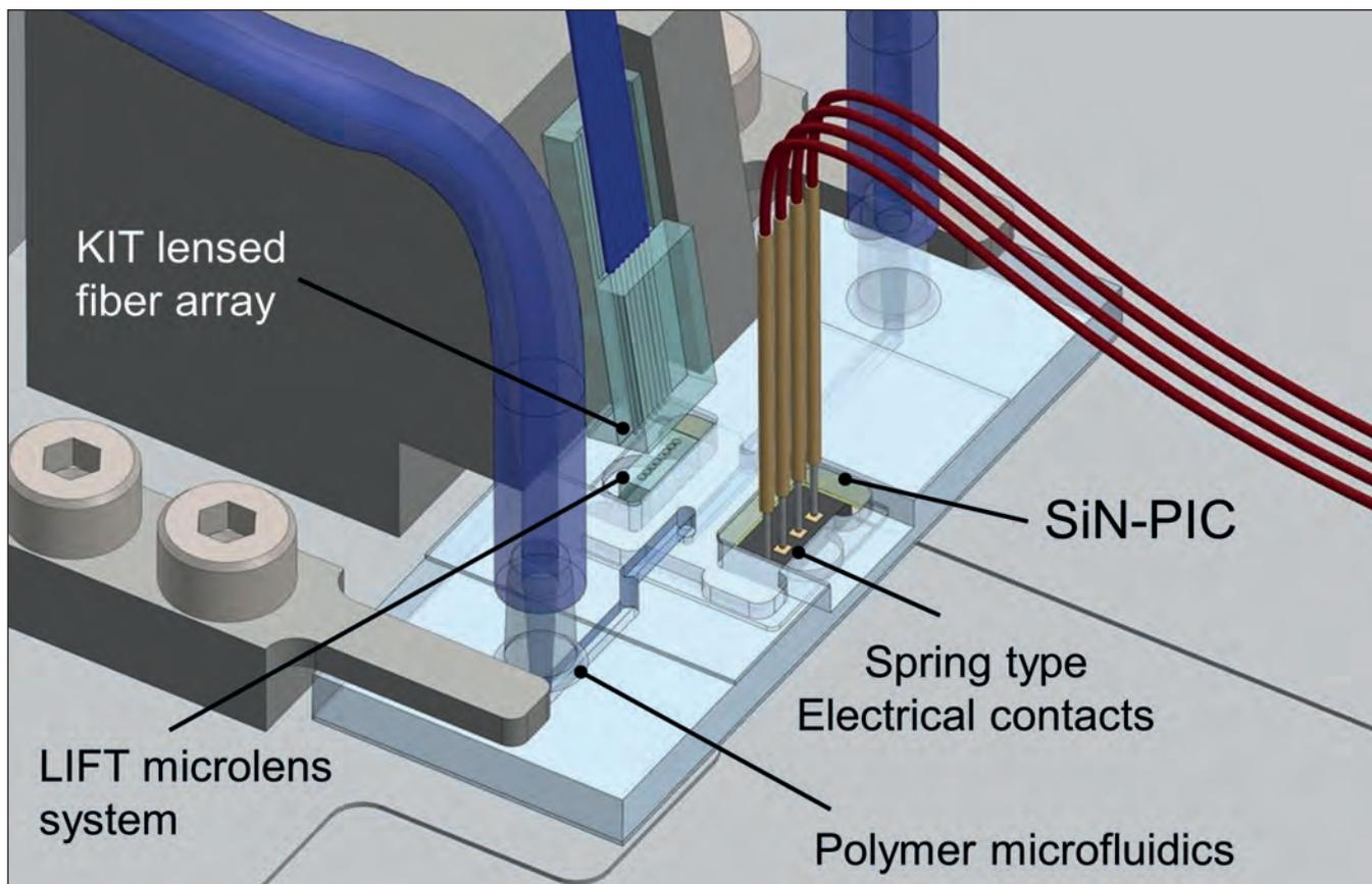
Figure 2. PIXAPP building blocks for free-space based disposable biosensors are ready for customized developments
