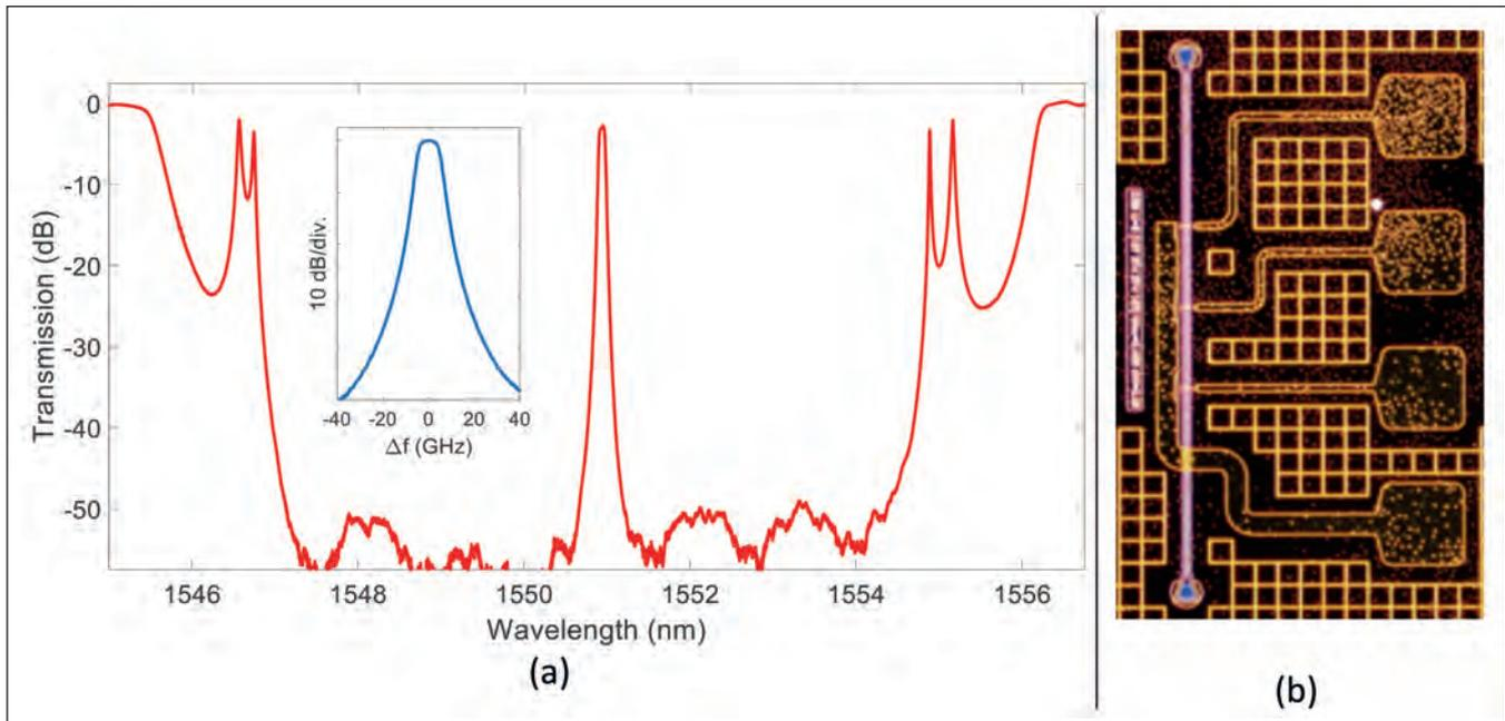
Figure 2: (a): Spectral transmission of a 3rd-order DFBR with a control signal applied to the MHs. The inset shows a close-up of the passband with a -3dB bandwidth of 10 GHz; (b): Micrograph of the fabricated sample consisting of the DFBR and metal pads and control lines for MHs.
