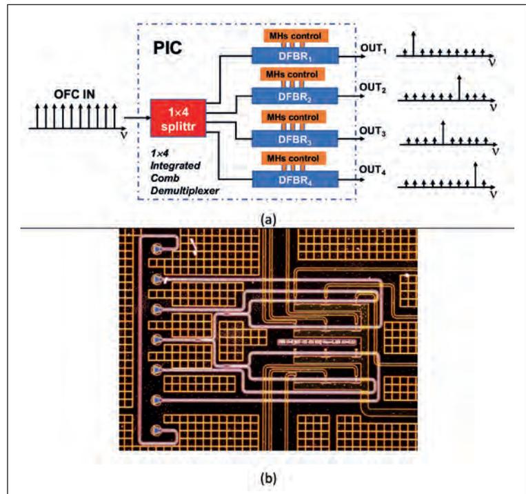
Figure 4: (a): Schematic operation of a photonic-integrated 1x4 OFC demultiplexer based on DFBRs; (b): Micrograph of fabricated device.
