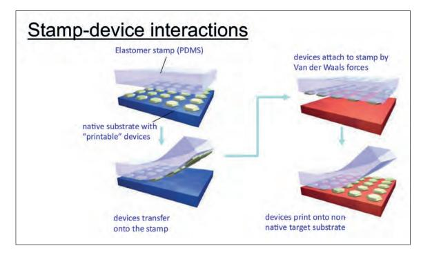
Figure 1: Basic process of micro transfer printing (MTP). Adapted from Meitl et al.<sup>1</sup>
