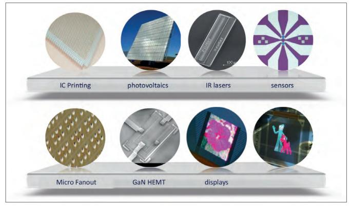
Figure 6: A list of technologies that have already benefited from MTP. Each image shows a device that was created using MTP.
