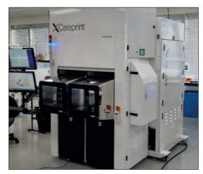
Figure 7: Automated MTP X-Celeprint tool capable of up to 200 mm wafer diameter fabrication.
