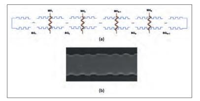
Figure 1. (a): Schematic top view layout of a Nth-order DFBR filter realized with a sidewall corrugated strip waveguide (b): Scanning electron microscope image of a fabricated grating. The devices were fabricated at the Inphotech Foundation facilities and at the James Watt Nanofabrication Centre at Glasgow University through the CORNERSTONE project.
