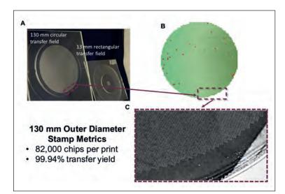
Figure 4: A) A PDMS stamp of a 130 mm circular (left) and 13 mm rectangular (right) transfer field. The 130 mm circular transfer field, matches a 150 mm wafer less a 10 mm edge, B) shows the device yield where pixels indicate successful prints and red pixels indicate failed prints. For 82,000 chips per print, 99.94% were successfully transferred. C) shows a close-up of the 130 mm circular transfer field at edge where the upper left portion is filled with PDMS stamp posts.
