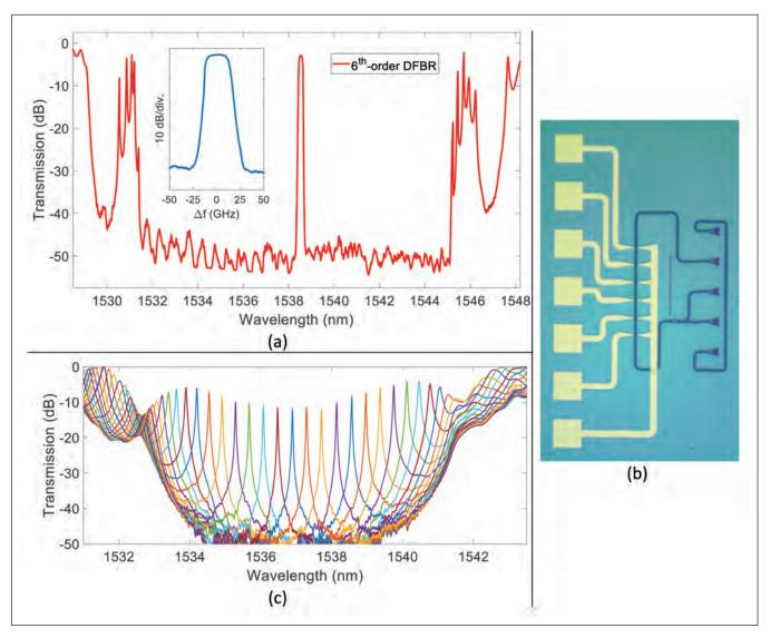
Figure 3: (a): Spectral transmission of a 6th-order DFBR; the inset shows a close-up of the passband with a -3 dB bandwidth of 25 GHz. (b): Micrograph of a fabricated 6th-order DFBR sample; (c): Tuning of the passband over the entire stopband for a 1st-order DFBR.
