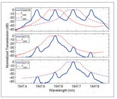
Figure 5. Normalized spectral transmission at the four output ports of the OFC demultiplexer when three DFBRs out of four are tuned through MHs for optimized response.
