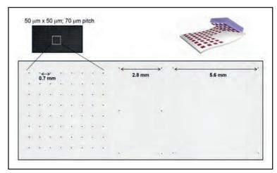
Figure 5: Example of fan-out capability for LEDs printed from a dense 70 micrometer source wafer (upper left) to a more sparsely populated target wafer of 0.7, 2.8, and 5.6 mm pitch (bottom). Adapted from Park et al. 3
