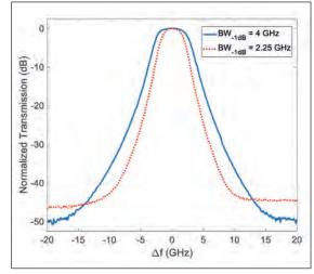
Figure 8. Different 3rd-order DFBR filter measured transfer functions also suitable for operation with 6.25 GHz comb spacing.
