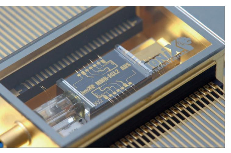
Figure 2. Narrow linewidth tunable laser based on hybrid assembly of an InP gain section and a tunable mirror made in TriPleX.
