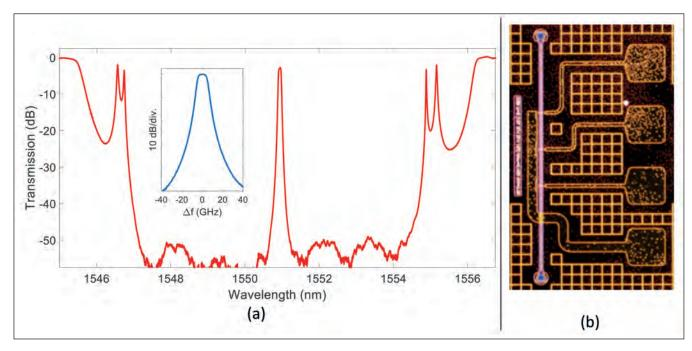
Figure 2: (a): Spectral transmission of a 3rd-order DFBR with a control signal applied to the MHs. The inset shows a close-up of the passband with a -3dB bandwidth of 10 GHz; (b): Micrograph of the fabricated sample consisting of the DFBR and metal pads and control lines for MHs.
