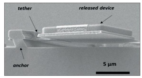
Figure 2: Scanning electron micrograph of a released device suspended above the open cavity by a tether and anchor.
