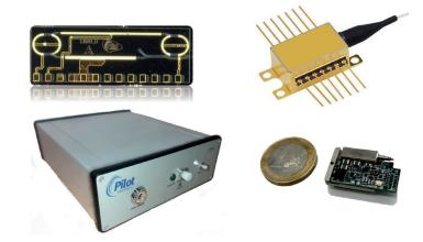
> Figure 1. Tuneable laser form factor offerings: Photonic Integrated Circuit (PIC), the laser cavity consists of a gain section providing optical gain in either the C or O bands, two ring sections that act as tuneable mode selectors through the Vernier effect, and a common phase section to allow finer tuning of the laser cavity mode; 14-pin butterfly package; OEM benchtop unit; nano-integrated tuneable laser assembly package.
