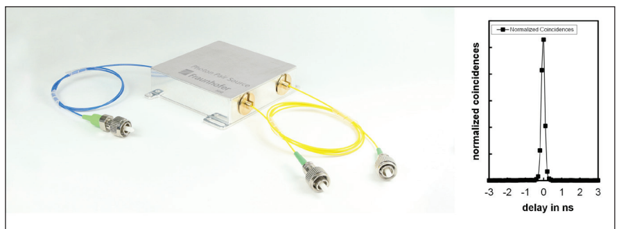
► Figure 4. Photon pair source module relying on the micro-optical bench in the PolyBoard platform.
