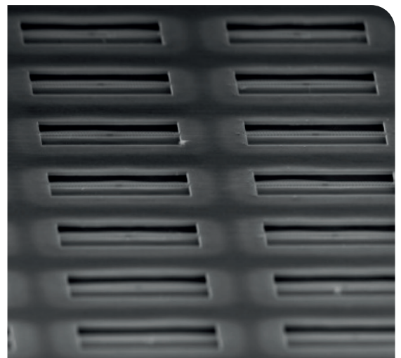
► Figure 2. A scanning electron microscope image of a fabricated one-dimensional photonic crystal laser array.
