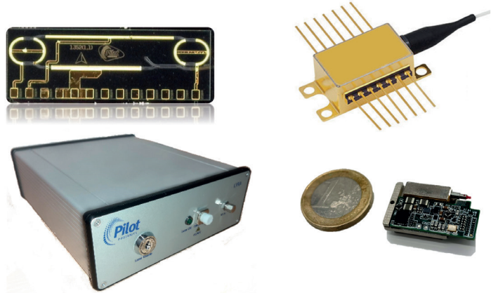
➤ Figure 1. Tuneable laser form factor offerings: Photonic Integrated Circuit (PIC), the laser cavity consists of a gain section providing optical gain in either the C or O bands, two ring sections that act as tuneable mode selectors through the Vernier effect, and a common phase section to allow finer tuning of the laser cavity mode; 14-pin butterfly package; OEM benchtop unit; nano-integrated tuneable laser assembly package.
