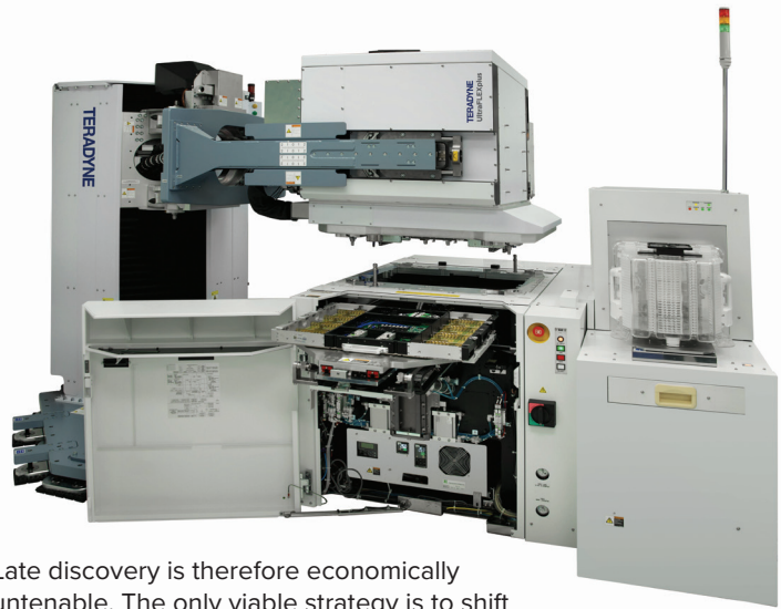
➤ Figure 1: Teradyne UltraFLEXplus with Photon 100 single-sided optical wafer probe cell (Courtesy of Teradyne)
