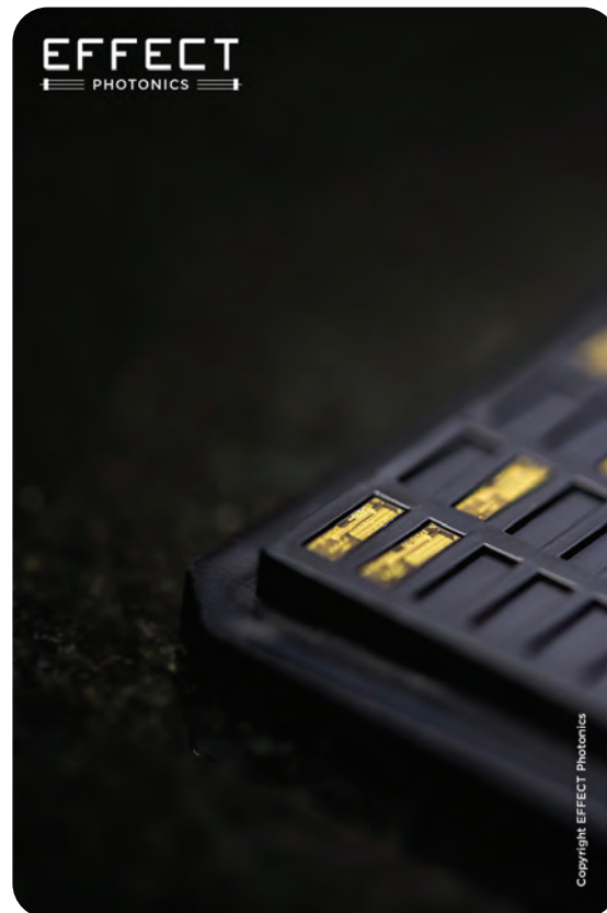
Figure 1: Fully integrated coherent PIC fabricate by EFFECT Photonics (courtesy of EFFECT Photonics)
