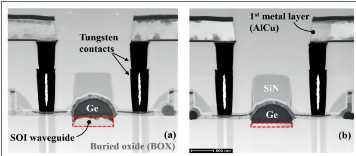
► Figure 1: TEM images of germanium photodiode (a) and electro-absorption modulator (b). Cross sections cut perpendicular to the light-incidence direction. As indicated by the red boxes the Si-region has been reduced from 220 nm to 100 nm for the electro-absorption modulator.
