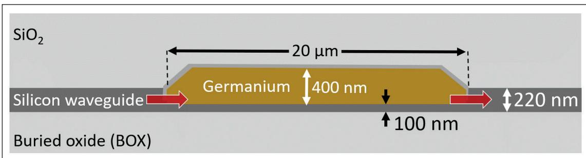
► Figure 2: Schematic longitudinal cut through the EAM to visualize the butt-coupling approach (not to scale).
