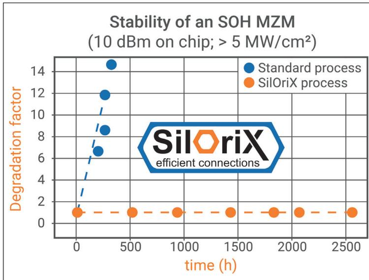
► Figure 3. Long-term photostability test of SilOriX SOH MZM. By intimate combination of material, process, and device development, SilOriX has managed to eliminate stability problems in its SOH devices, that were long perceived a roadblock towards industrial exploitation of the technology. The devices under test were operated for more than 2500 hours at an on-chip power of 10 mW, without any sign of photodegradation.
