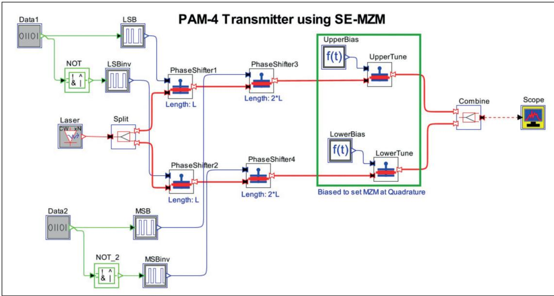
➤ Figure 1. Schematic of a PAM-4 transmitter using SE-MZM
