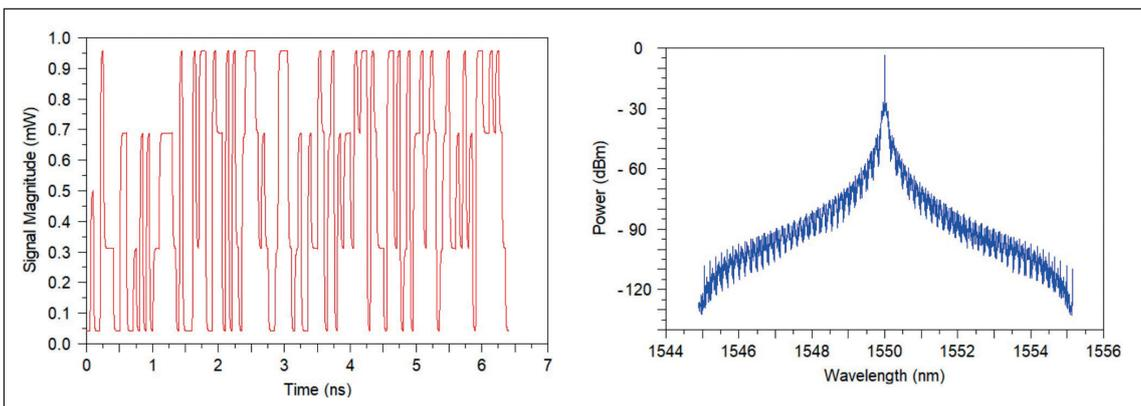
➤ Figure 2. SE-MZM PAM-4 transmitter output signal (left) and spectrum (right).
