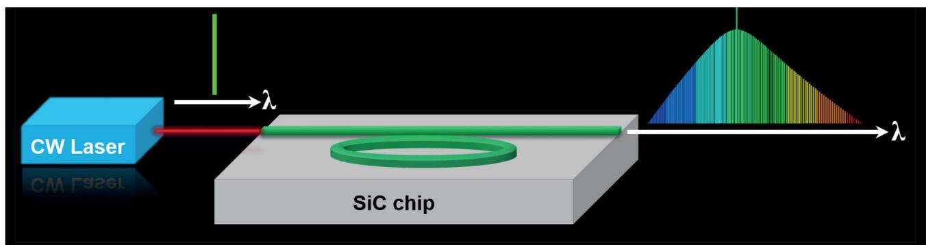
➤ Figure 2. SiCOI OFC generated from a microring resonator.
