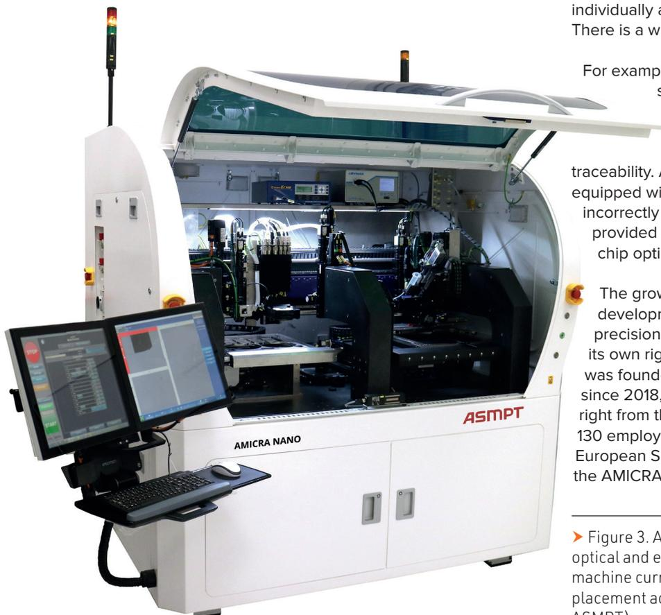
► Figure 3. AMICRA NANO: The bonder for processing optical and electronic components. The most precise machine currently on the market operates with a placement accuracy of  $\leq \pm 0.2 \mu\text{m}$  at 3 sigma. (Image: ASMPT).
