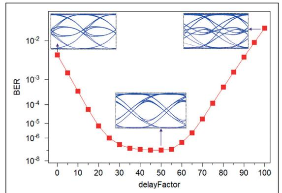
➤ Figure 8. Bit error rate (BER) as a function of driving time delay.
