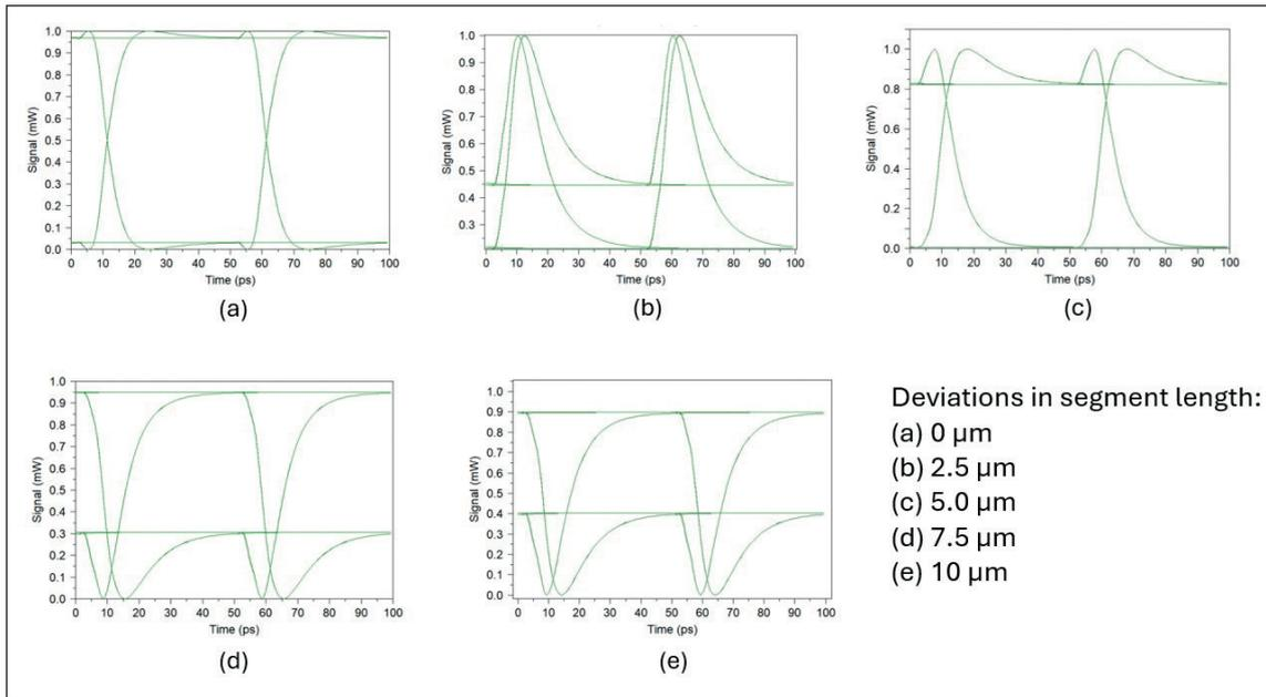
► Figure 5. Optical eye diagrams at the transmitter output.
