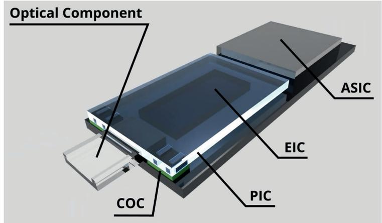
➤ Figure 1. Example of a Chip-on-Carrier (COC) embedded in CPO: A laser COC is placed on a PIC wafer together with an electronic IC (EIC). This is then combined with an optical component and the application-specific IC (ASIC) on the substrate to form an optical engine (OE). (Image: ASMPT)
