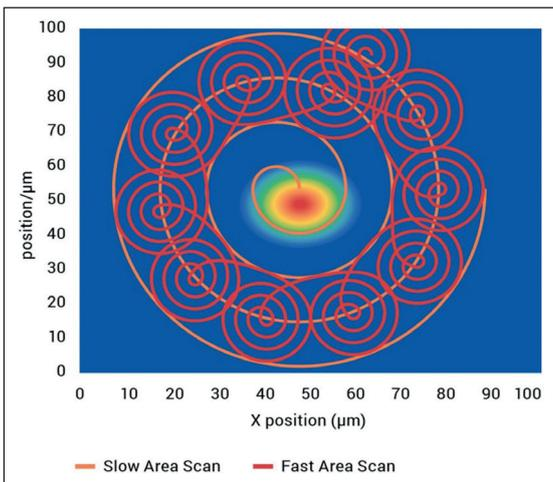
➤ Optical feedback is the key to automated alignment. A fast, traditional way of finding first light followed by a gradient search for optimum coupling efficiency is shown above – a double spiral scan using a hexapod/piezo approach. The hexapod runs a coarse spiral scan (coarse meaning single digit microns), while the piezo stage fills in the gaps with high-speed sub-micron scans. Both fine and coarse scans can be executed simultaneously. (Image courtesy PI)
