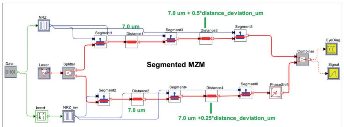
► Figure 4. Schematic of a PAM-2 transmitter using SE-MZM.
