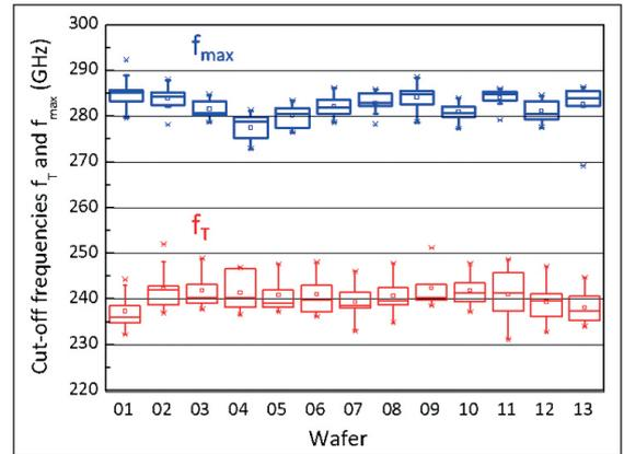
➤ Figure 6: Box-plots of unity gain frequency  $f_T$  and of maximum oscillation frequency  $f_{\text{max}}$  measured on 13 wafers from one lot, 9 chips measured on each wafer.
