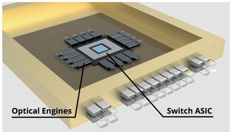
➤ Figure 2. CPO with external laser SFP (ELSFP) as the signal carrier. Laser light sources are placed externally at the faceplate of the SFP, and modulations are kept at the CPO. Fibre connections replace the original copper traces. (Image: ASMPT).
