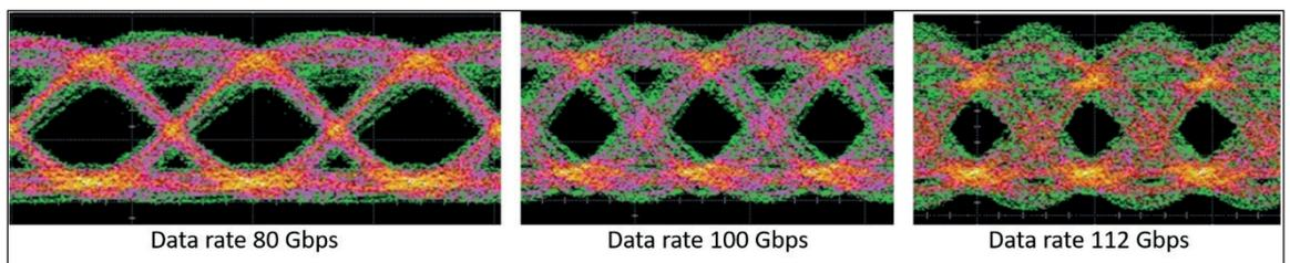
► Figure 4: Eye diagrams of RF-probed germanium EAM at data rates of 80, 100, and 112 Gbps. The dynamic extinction ratios are 2.9 dB (80 Gbps), 2.75 dB (100 Gbps), and 2.3 dB (112 Gbps) with four-tap linear equalization on the receiver side.  $V_{bias} = -1.5$  V and an AWG output signal of  $2.3 V_{pp}$ .
