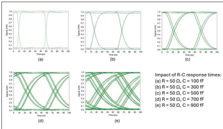
➤ Figure 11. Optical eye diagrams at the transmitter output.
