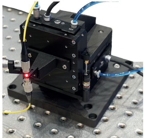
➤ A compact, multi-axis air-bearing based photonics alignment system. Advantages of air bearings are frictionless, high-speed motion with virtually unlimited lifetime as well as the lack of particle generation. (Image courtesy PI).
