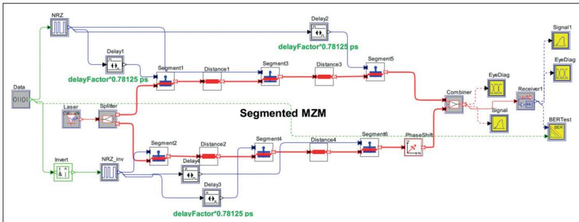
► Figure 6. Schematic of a PAM-2 transmitter using SE-MZM.
