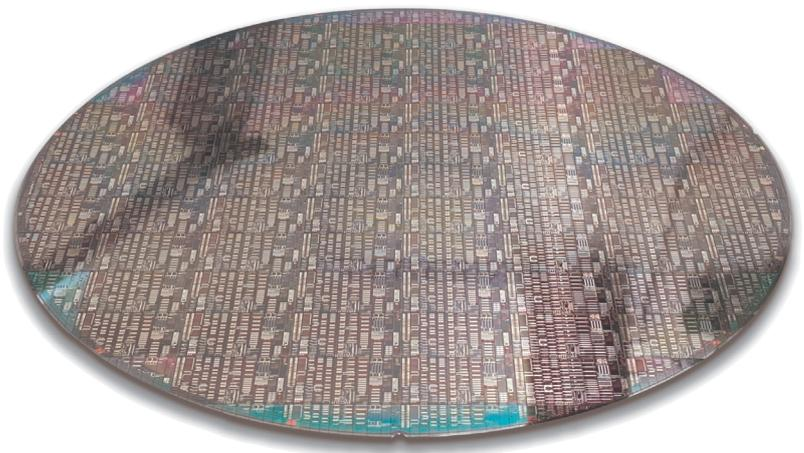
► Figure 2. An 8-inch SOH wafer fabricated by SiOriX and its partners, carrying more than 25,000 SOH modulators along with a wide range of high-end silicon photonic circuits for various applications in optical communications, ultra-broadband signal processing, and optical metrology.
