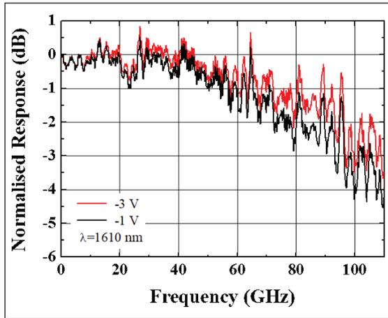
► Figure 3: Normalized frequency response of electro-absorption modulator at wavelength of 1.6 μm at a bias of -1 V and -3 V for an optical input power of  $P_{in} = 6$  dBm at fibre tip, estimated on Keysight 110 GHz LCA.
