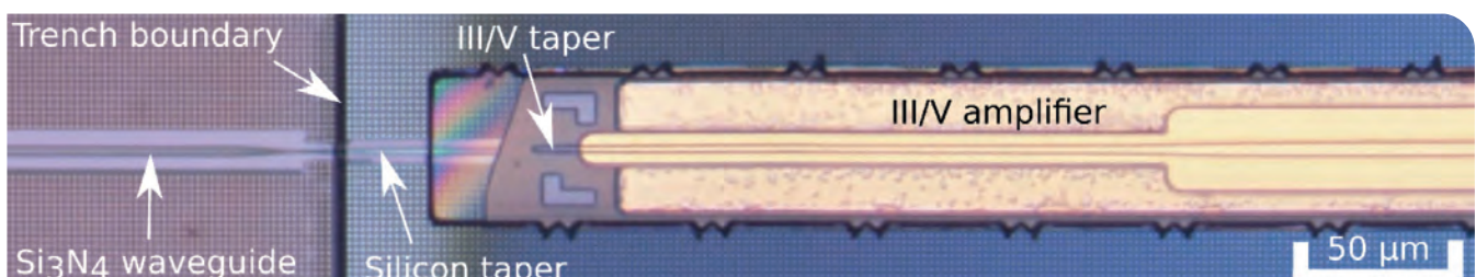
Figure 2. Microscope image of the micro-transfer printed coupon on top of the two-stage taper coupling structure.
