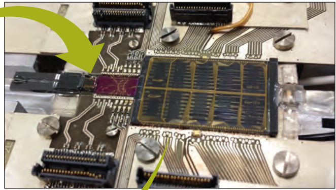
➤ Figure 3: The importance of a vertically integrated approach to photonic module design. An early version of a photonic OBFN (top left) included a SiN PIC but used common off-the-shelf components to connect it to modulators and electronics, resulting in a very bulky and fragile device. Using a InP PIC modulator, hybrid integration allowed for the construction of a much smaller device (top right). However, using wire bonds to connect the chips and not codesigning its electronics meant that the device was still fragile and bulky. By co-designing the PICs, their assembly, and its electronics and interconnects, the device achieved an assembly with thermal dissipation, mechanical stress relief, and packageability (bottom). At the same time, the device is cheaper to manufacture, easier to characterize, and is more powerful.
