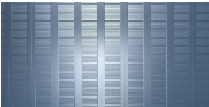
➤ Figure 4: Wafer-level structured substrate with engineered V-grooves.
