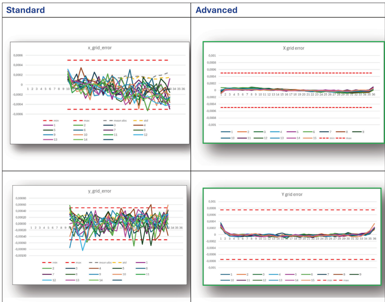
➤ Figure 5: Wafer test result showing Gaussian distribution of grid error.
