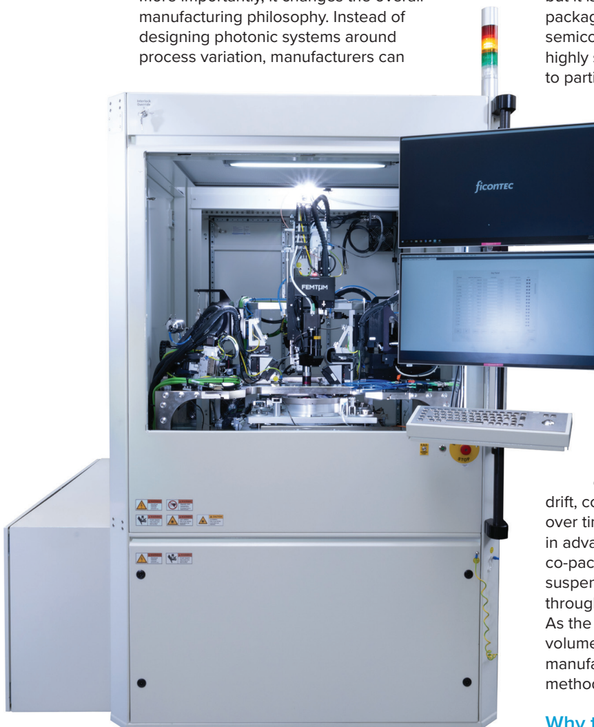
➤ Figure: Femtum's laser trimming and cleaning solution integrated into a ficonTEC equipment.
