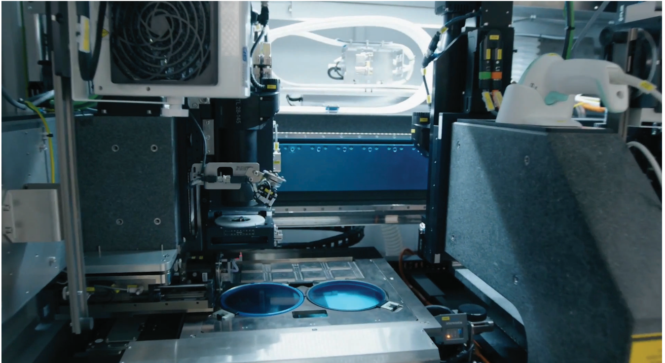
➤ A look inside the AMICRA NANO: Source stage, flip unit and bond head support the sub-micron precision required to evaluate optical alignment strategies and process windows during early CPO development. Image credits: ASMPT
