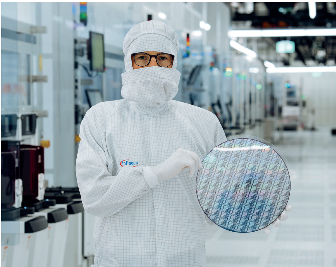
➤ A technical engineer in the cleanroom at Infineon Technologies in Villach, Austria, holds a 300 mm GaN-on-silicon wafer.
