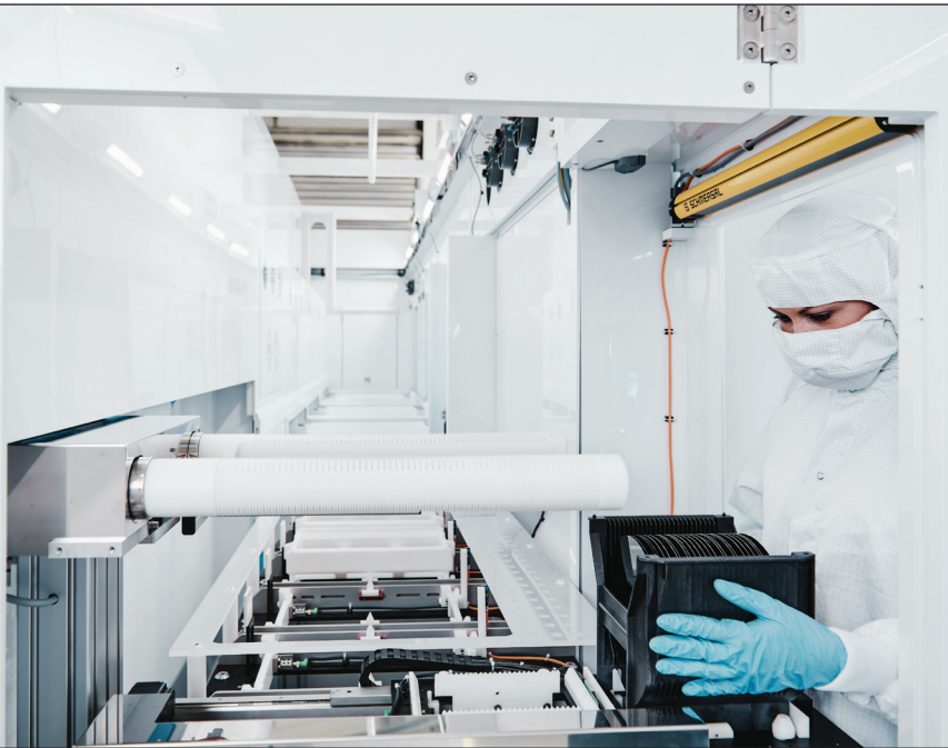
Fully automated A-Series wet bench from AP&S
