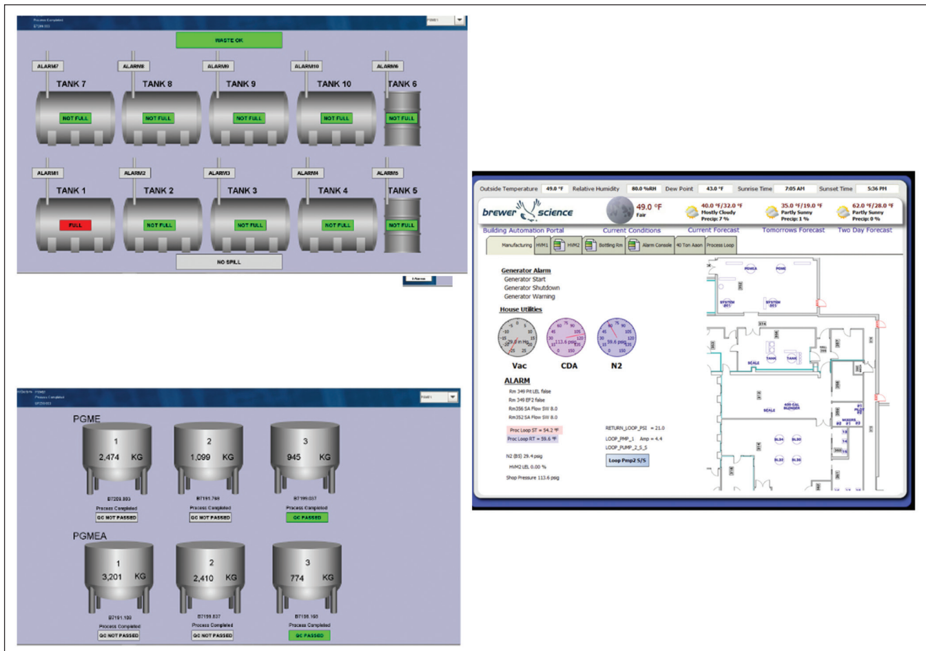
Figure 2: Factory automation portal. In this example, tank 1 has an issue that needs to be addressed).
