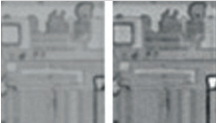
Figure 2. Acoustically bright defect at right was not found by standard imaging.
