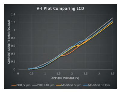
Figure 1: V-I plot comparing LCD of POR condition against modified condition
