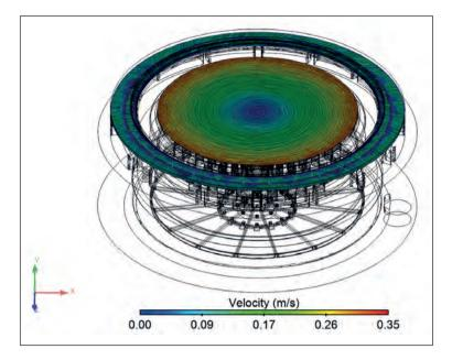
➤ Figure 2: CFD image of electrolyte at wafer surface applications at >32nm node.
