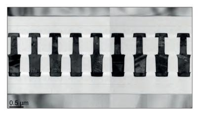
Figure 2: Wafer-to-wafer hybrid bonding at 700nm pitch (as presented at 2021 IEDM).
