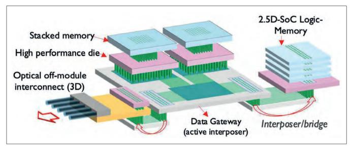
➤ Figure 1: Abstracted view of a possible future high-performance system. High-performance die with 3D-SOC stacked memory are implemented on an active interposer chip which acts as a data gateway and connects in a '2.5' fashion with local high bandwidth memories and optical transceiver modules (as presented at 2021 IEDM).
