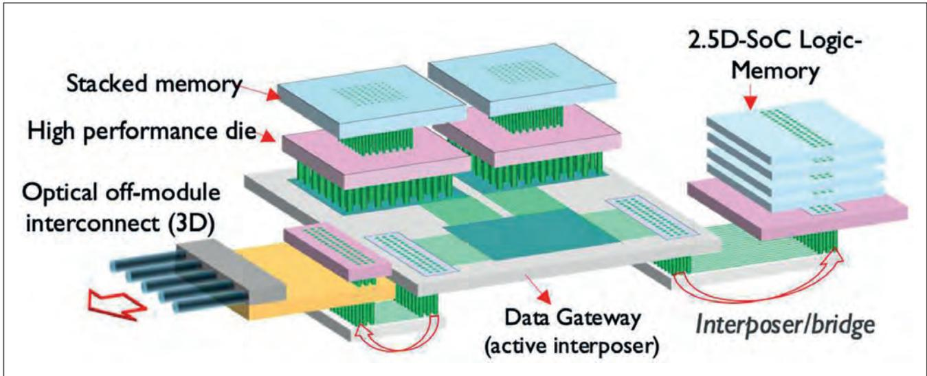
➤ Figure 1: Abstracted view of a possible future high-performance system. High-performance die with 3D-SOC stacked memory are implemented on an active interposer chip which acts as a data gateway and connects in a '2.5' fashion with local high bandwidth memories and optical transceiver modules (as presented at 2021 IEDM).
