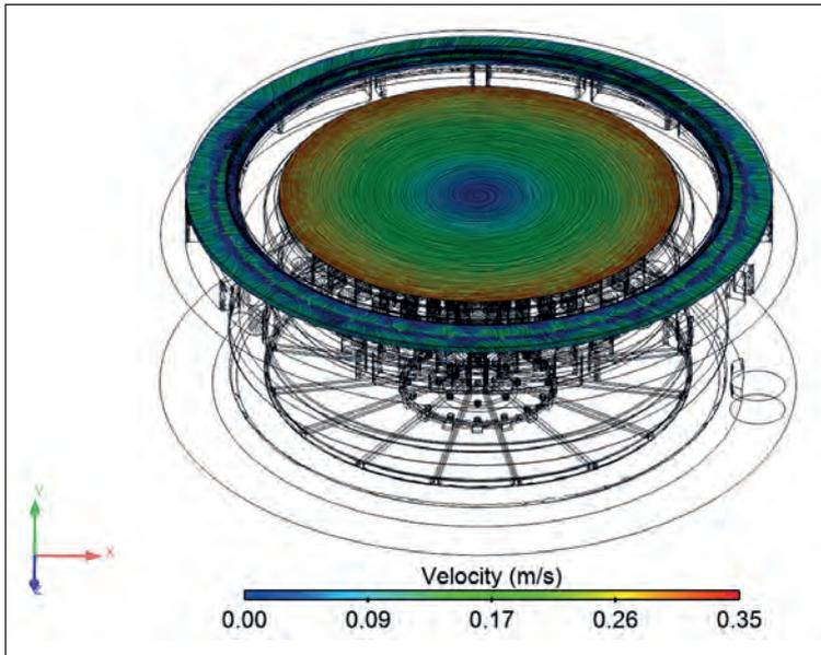
► Figure 2: CFD image of electrolyte at wafer surface
