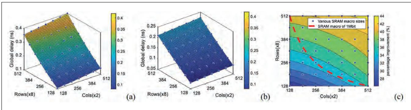
➤ Figure 4: Global routing delay (read access) of SRAM macro at various macro rows and columns. (a) FS; (b) BS and (c) from FS to BS improvement. The macro size ranges from 128\*128\*16=256kbit to 515\*512\*16=4Mbit (as presented at 2021 IEDM).
