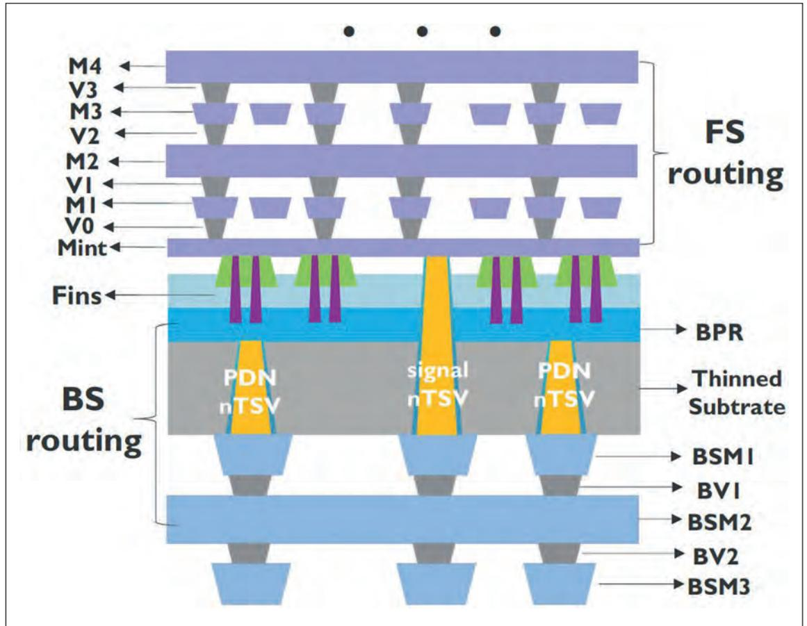
macros to be placed in the top die, while the logic is placed in the bottom die. On the technology side, this can be realized by bonding the active frontside of the 'logic wafer' to the active frontside of the 'memory wafer' by using a low-temperature wafer-to-wafer bonding technique. In this configuration, the original backsides of both wafers now reside on the outside of the 3D-SOC system.
