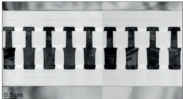
➤ Figure 2: Wafer-to-wafer hybrid bonding at 700nm pitch (as presented at 2021 IEDM).
