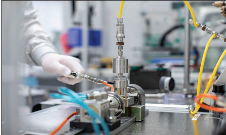
Figure 2. Advanced UHP ALD valve designs like that found in the Swagelok ALD20 UHP valve are enabling greater thermal stability, higher flow rates, and increased innovation in semiconductor wafer manufacturing.
