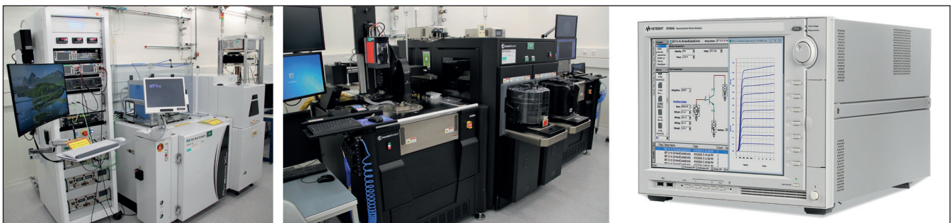
➤ Figure 6: Electrical measurement technology at the Fraunhofer Center (left: automatic wafer prober, middle: semi-automatic wafer prober, right: semiconductor parameter analyzer). ©Fraunhofer IPMS
