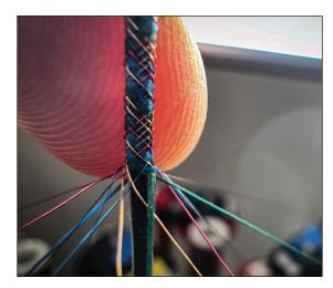
macroscopic version of the fiber computer, called a preform, that contains each connected microdevice. This preform is hung in a furnace, melted, and pulled down to form a fiber, which also contains embedded lithium-ion batteries so it can power itself.
