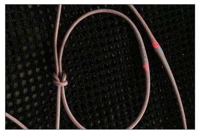
> This single, elastic fiber contains a series of microdevices, including sensors, a microcontroller, digital memory, bluetooth modules, optical communications, and a battery, making up all the necessary components of a computer. Credit: Yoel Fink, edited by MIT News
