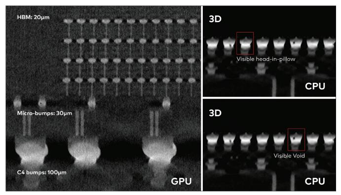
Figure 2: Left, virtual slice of a reconstructed X-ray scan of a commercially available GPU with 100µm C4 bumps, 30µm microbumps and 20µm high bandwidth memory bumps. Right, virtual slice of a reconstructed X-ray scan of a commercially available CPU with ca 65µm C4 bumps. All image property rights remain with Comet Yxlon and images are not to be copied or distributed
