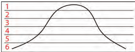
Figure 3. Gating the return echoes produced six depth-specific acoustic images.
