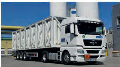
Compressed gaseous hydrogen (CGH 2 )
