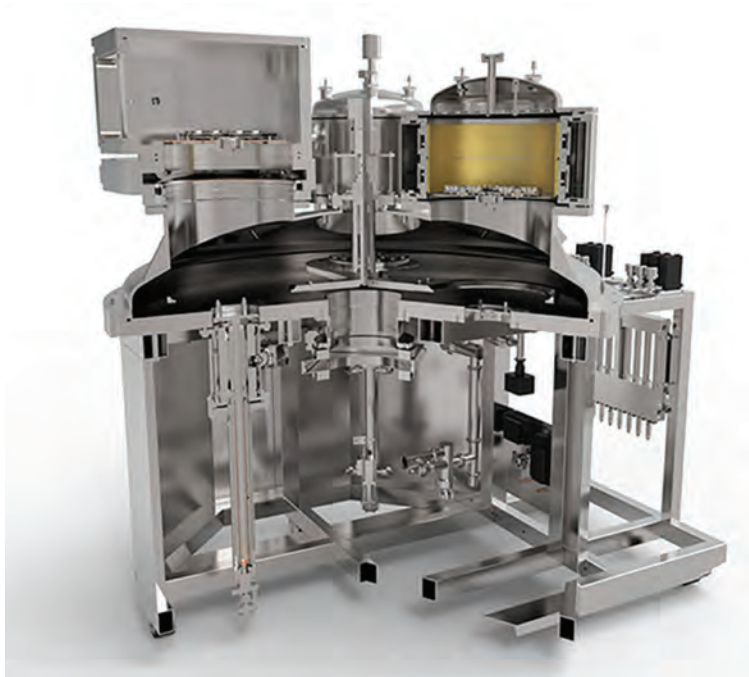
Figure 2. Cutaway view of the system layout showing the load lock on the left and sputtering cathode on the right.
