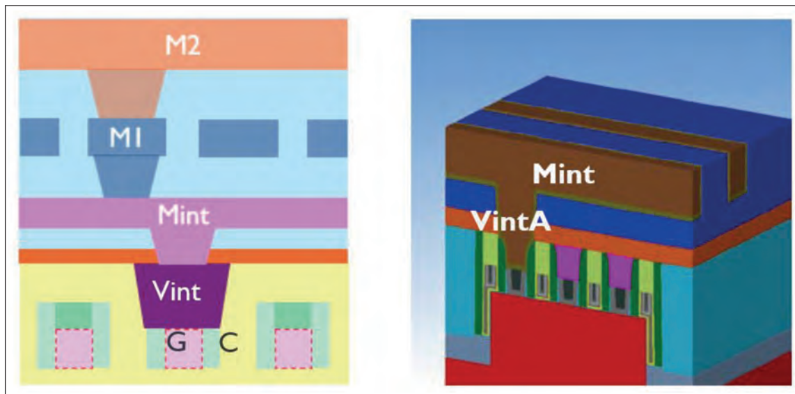
(Left) MOL stack and (right) self-aligned gate contact.
