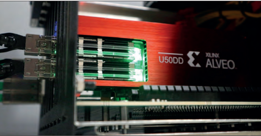
Figure 5: SMV Subscriber Accelerator application over Alveo in a dedicated PCIe expansion chassis.
