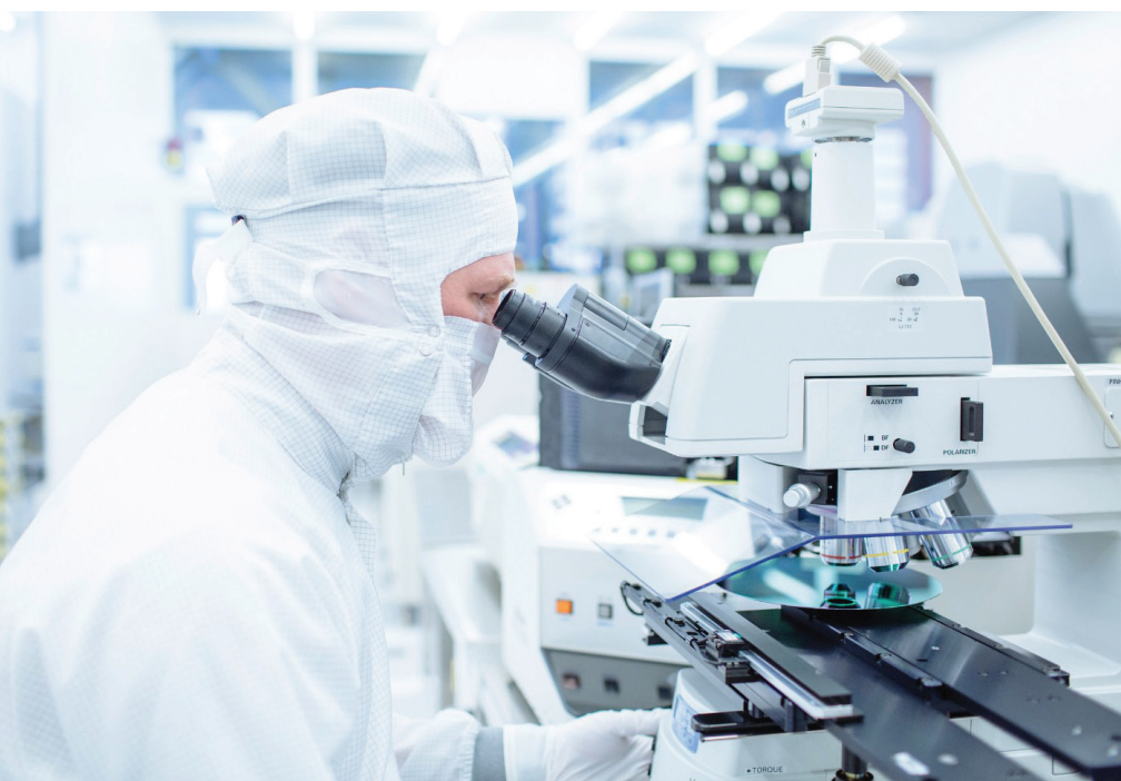
➤ Quality inspection in the wafer manufacturing process. © Fraunhofer IPMS
