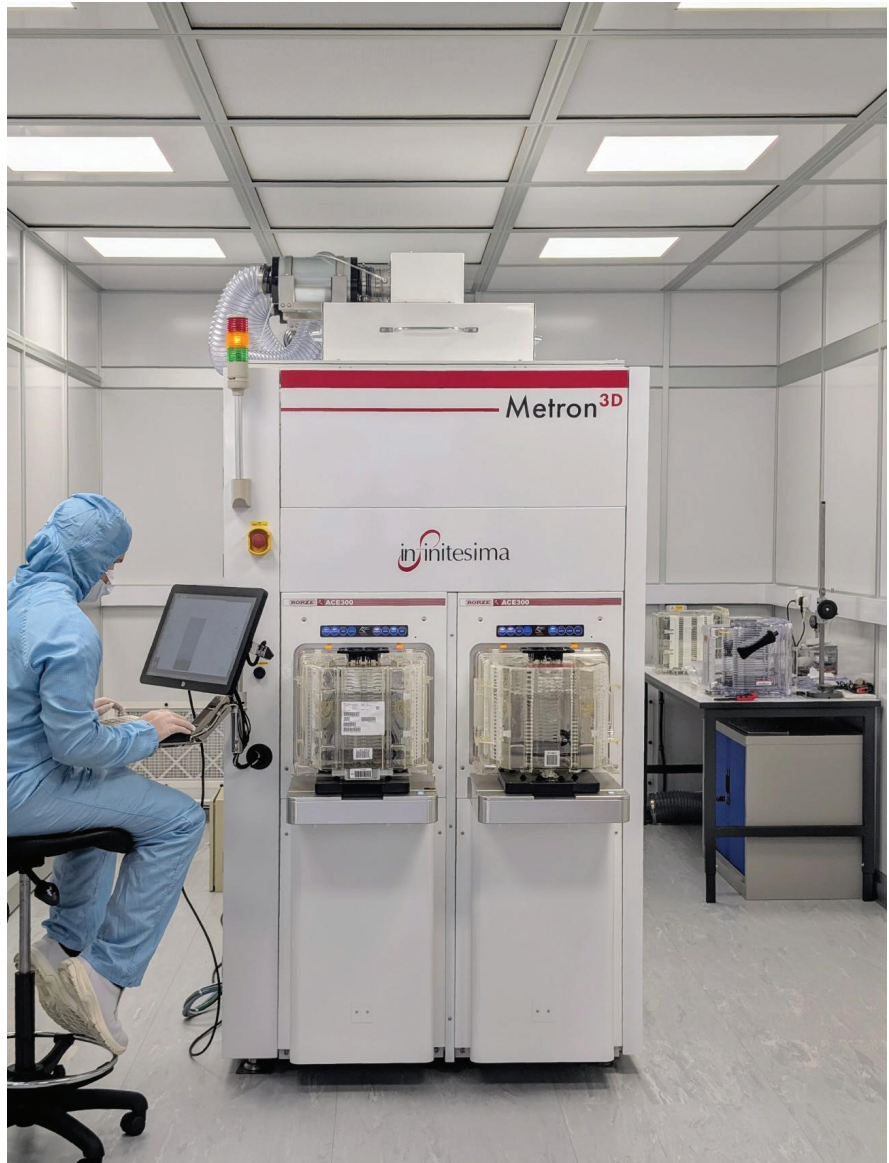
➤ Infinesima’s Metron3D metrology system is designed to measure challenging nanoscale structures in semiconductors at high speed. [Infinesima]
