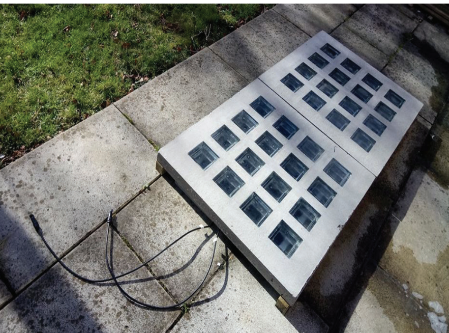
Solar sidewalk (C) test bed
