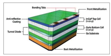
Figure 1. The GalnP/InGaAs/germanium lattice-matched, triple-junction cell is monolithic device that is grown on a germanium substrate.
