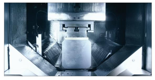
factor is that, even with the thinnest wires, the sensitive control reliably maintains the extremely fine line between optimum yield and the risk of a wire break: the wire tension remains constant up to 0.5 N. Without exerting any additional stress on the wire, the cyclic acceleration and braking processes can be configured more dynamically and in addition, a higher cutting speed can be maintained – up to 30 m/s.
