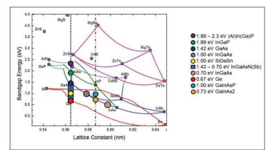
Figure 4: Bandgap and lattice constant for a number of semiconductor materials, with the III-V materials of particular interest for multi-junction cells noted.
