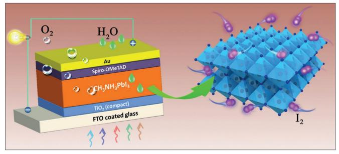
The schematic drawing showing that various factors (e.g., moisture, oxygen, light illumination, applied electric field, etc.) during the operation of MAPbl3 perovskite solar cells can generate iodine, which leads to degradation of solar cells.
