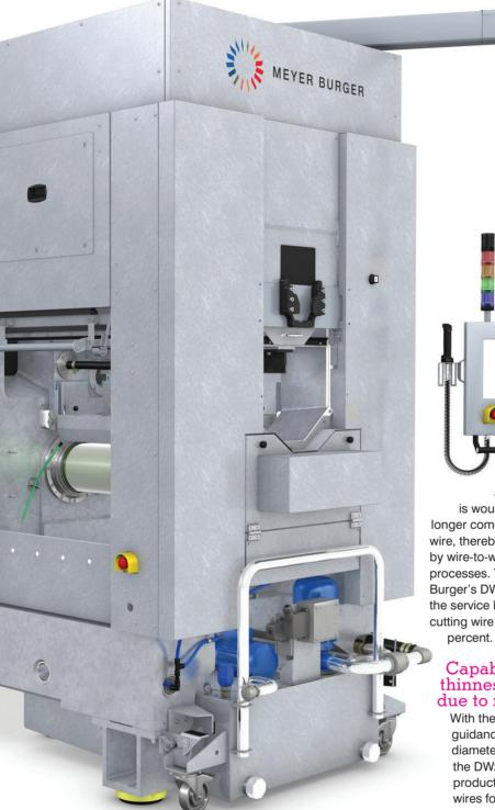
More and thinner wafers in a shorter time and with a lower consumption of diamond wire: Meyer Burger's DW288 Series 3 diamond wire saw combines a patented wire management system, optimized distances and diameters of the wire guiding rollers, and a consistently optimized automation, to create a highly productive overall package with a secure future.
